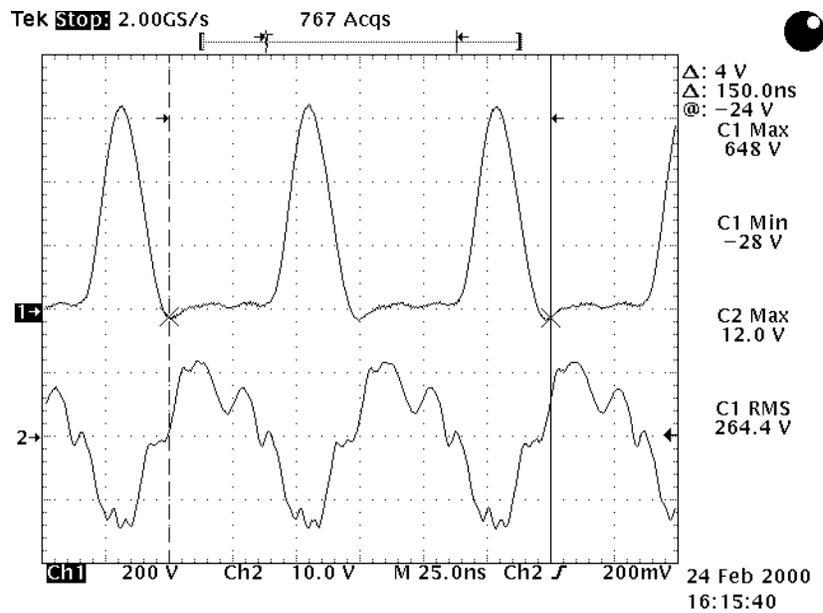
**Figure 5 2x ARF448 waveforms.  $P_o = 600W, \eta = 90\%$ .**
