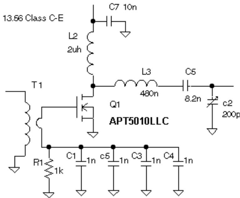
**Figure 3 Schematic as Built – 1kW @ 13.56  $\eta$ =89%**
