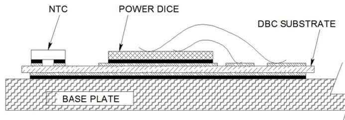
Fig 1: NTC thermistor location on a substrate
