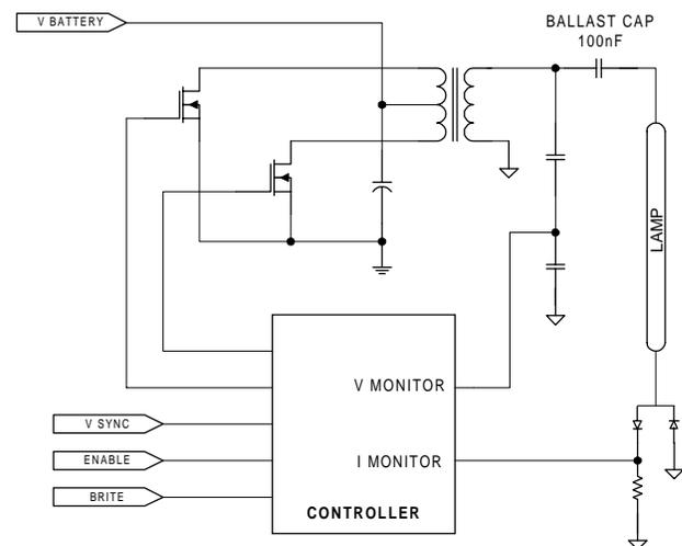
Figure 2: Direct Drive Simplified Circuit
