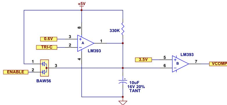
**Figure 14: Open Circuit Time Out**
