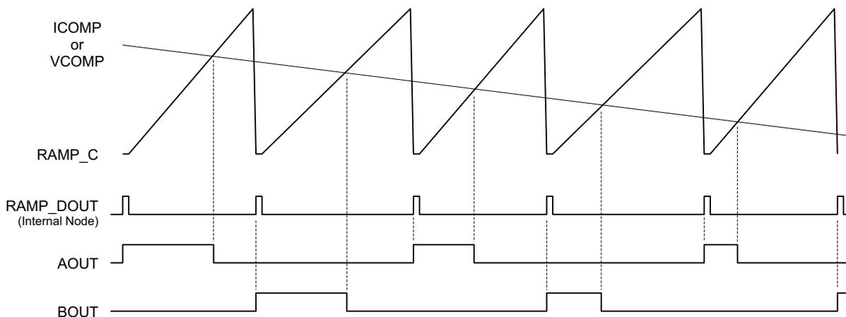
Figure 7: Direct Drive PWM Regulation Timing Diagram
