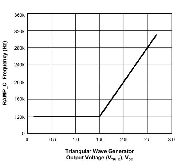
Figure 5: RAMP\_C Frequency vs.  $V_{TRI\_C}$
