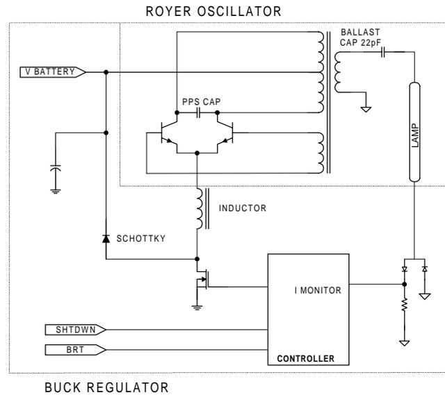
Figure 1: Buck/Royer Simplified Circuit
