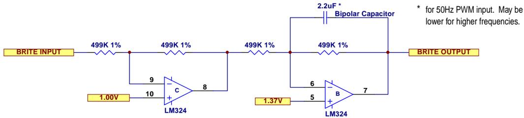
**Figure 13: Brite Input Conditioning Circuit**
