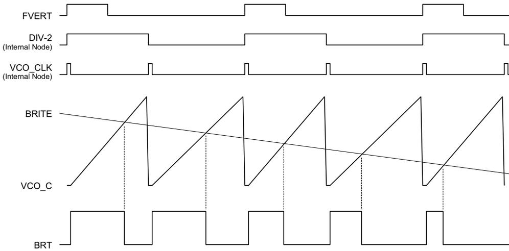
Figure 4: Digital Dimming Timing Diagram
