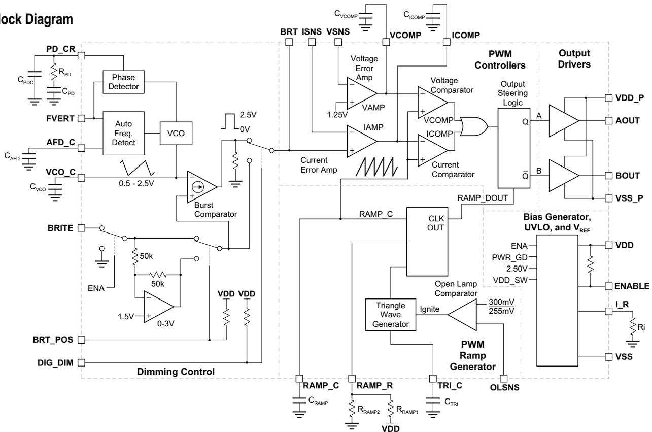
Figure 3: LX1686 Simplified Block Diagram
