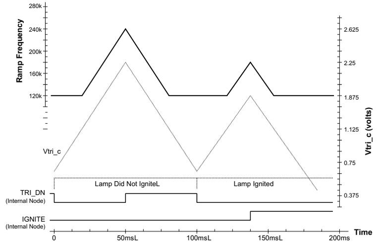
Figure 6: Lamp Ignition Timing Diagram
