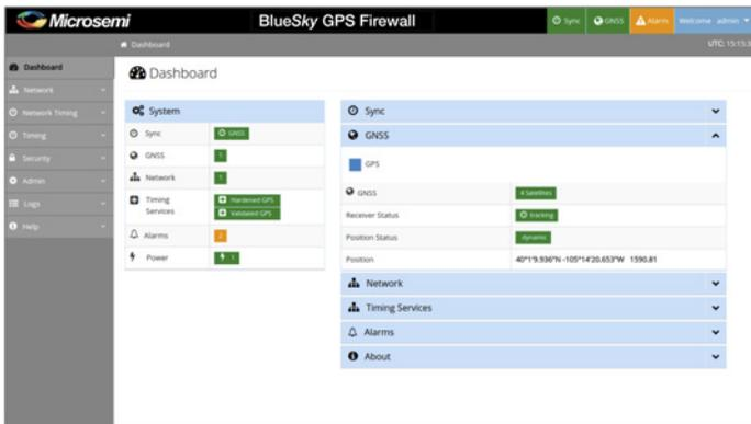
The BlueSky GPS Firewall provides users control from a web-based graphical interface and the ability to update data validation rules
