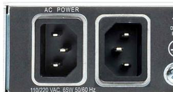
The dual AC power supplies provide hitless switching from one power supply to the other in the event of a power outage on one circuit of a dual circuit power scheme, or a power supply failure. The supplies are continuously monitored and an SNMP trap is sent, in the event one of them fails. For extra level of assurance, the power cord(s) supplied with the SyncServers have locking rear IEC 60320 connectors that prevent accidental decoupling.
