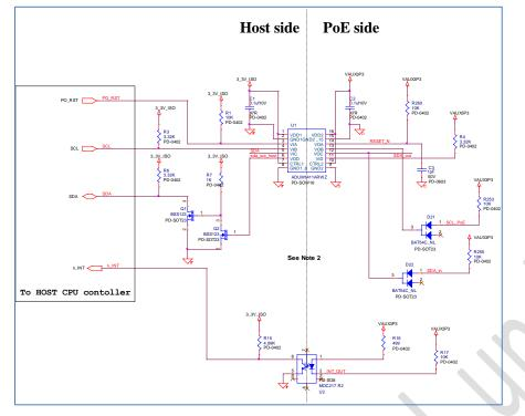
Figure 7: Digital Isolator + interrupt isolator
