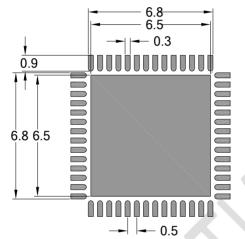
Figure 22: Thermal Pad Array Footprint (CS)
