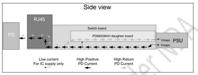
Figure 16: Component Identification for PD69208AH Circuitry
