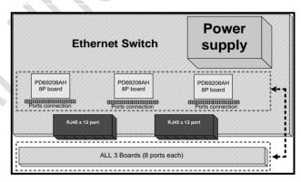
Figure 18: PoE DB Circuitry Inside the Switch
