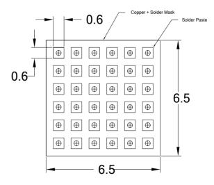
Figure 25: Bottom Solder Printing Mask (PS)
