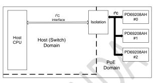
Figure 2: 12-port Configuration block diagram
