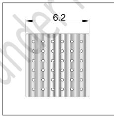
Figure 23: Thermal Pad Array Footprint (PS)
