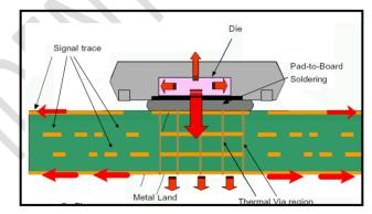
Figure 21: Heat Dissipation in PC
