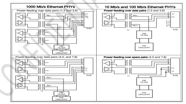
Figure 14: Output Ports Design Details
