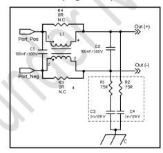
Figure 13: Recommended EMI Filter
