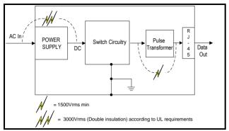
Figure 10: Standard Switch Circuitry
