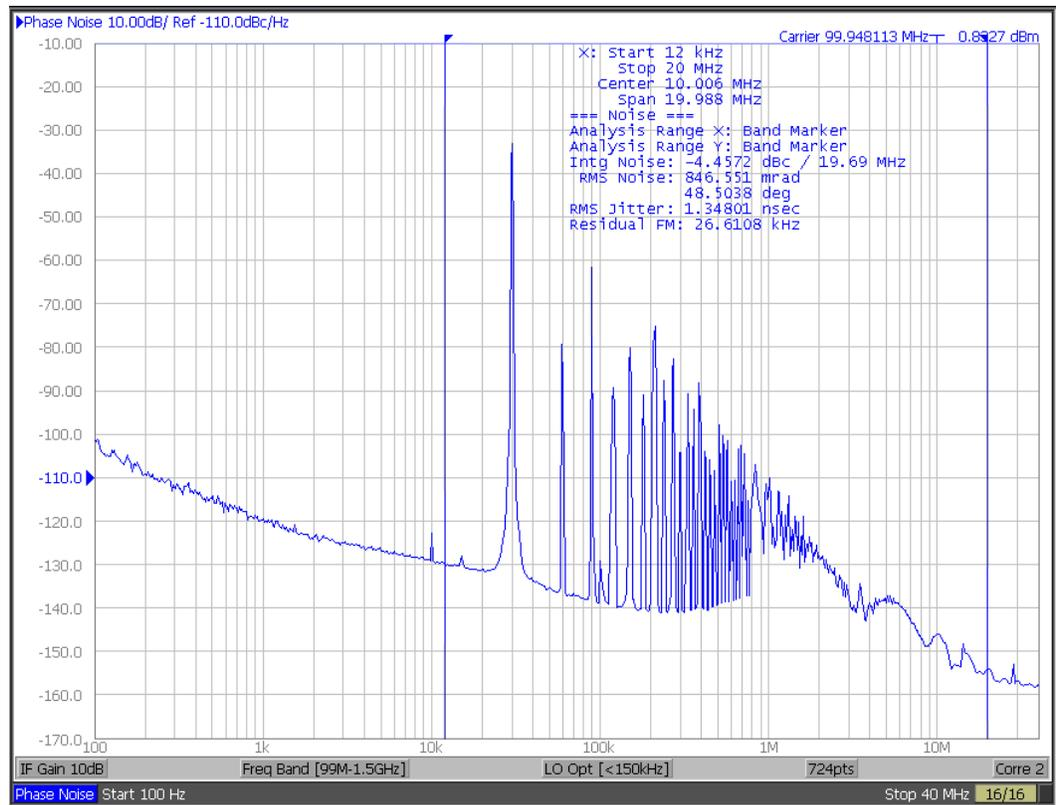
**Figure 5 - Phase Noise of 100MHz Signal Modulated with 30kHz Triangle Wave for 0.1% Spread**
