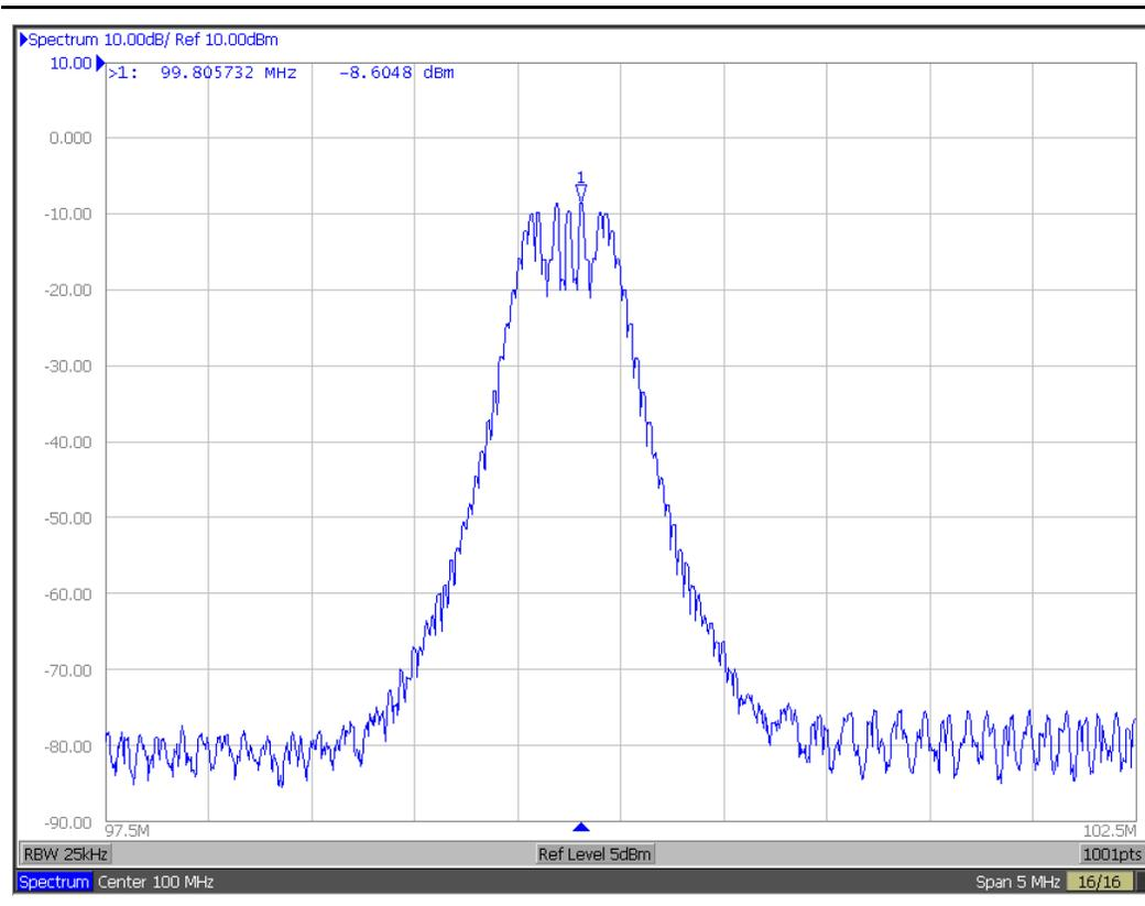
**Figure 2 - Spectrum of 100MHz Signal Modulated by 30kHz Triangle Wave with 0.5% Down-spread**
