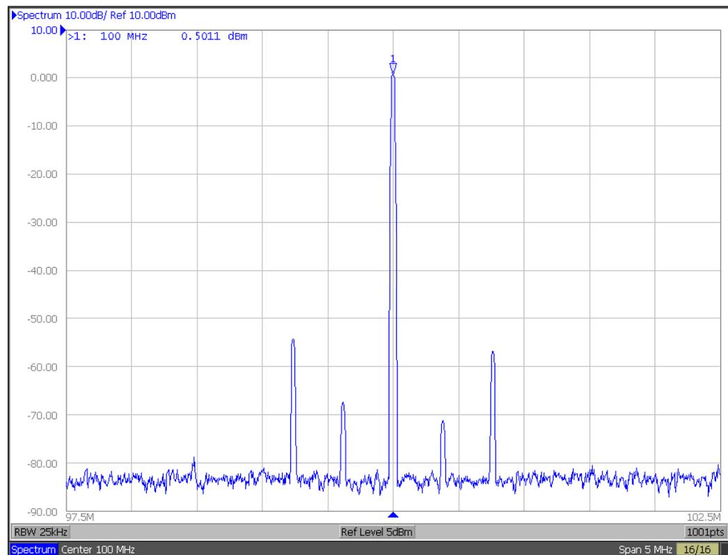
Figure 1 - Typical Spectrum for 100MHz Signal
