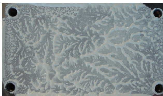
Picture2: Grease on the heat sink after removing the module
