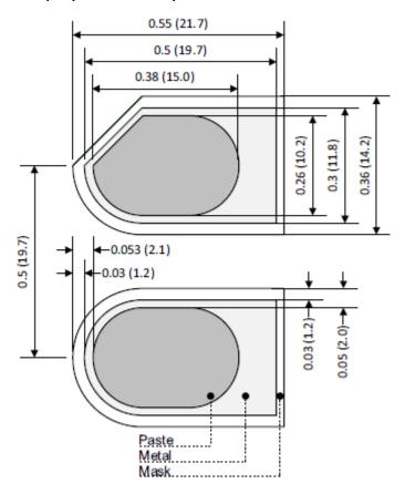
**Note:** The CM has latitude to modify the solder paste stencil for manufacturability reasons. The solder paste stencil shall cover 65% to 80% of the thermal pad and must not allow solder to be applied to the thermal vias under the QFN package using any method they deem appropriate. Any design should be subject to system validation and qualification prior to commitment to mass production of field deployment. Use a 5 mil stencil.
