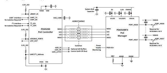
**Note:** For complete reference design, consult Microsemi AN211 Designing an IEEE 802.3af/802.3at/802. 3bt-Compliant PD69208 48-Port PoE System (Document Number: PD-000300282).
