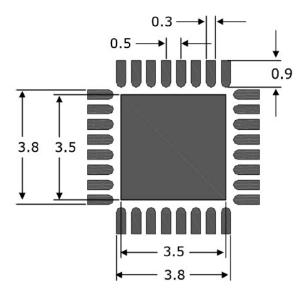
Figure 7 • PD69200 Top Layer Solder Paste and Vias PCB Layout for Thermal Pad Array
