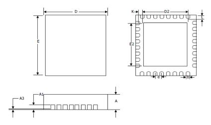
The following table lists the dimensions and measurements of the PD69200 package.
