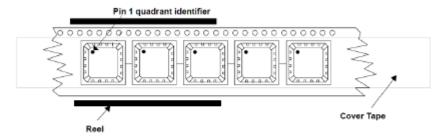
Pin-1 Orientation of QFN Packages
