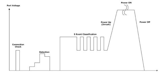
Figure 22 • Typical IEEE802.3bt Port PoE Voltage Diagram
