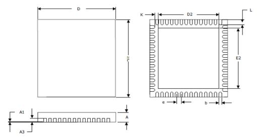
The following table lists the dimensions and measurements of the PD69208T4 package.
