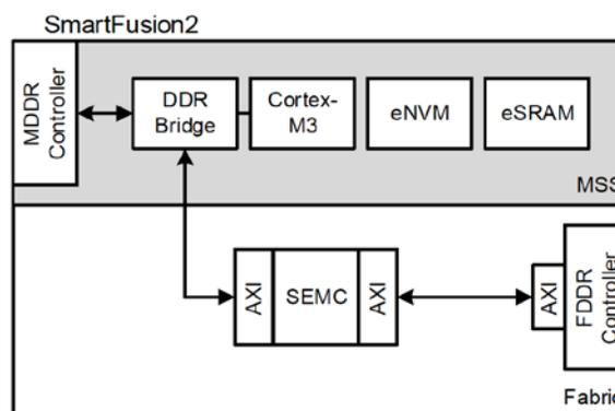
This is one example of using the SEMC to protect processor external memory accesses. More generally, the core may be used to protect any memory access bridged through the SEMC for both low latency and high-throughput applications.
