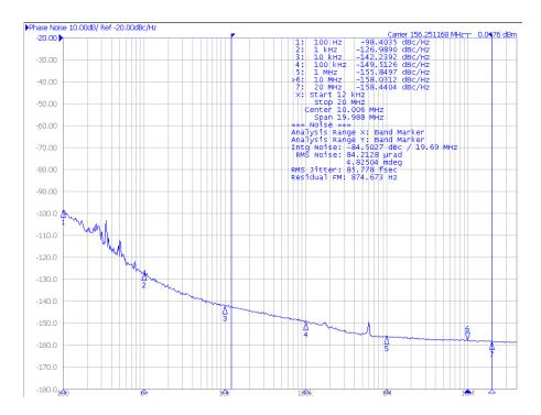
Figure 3: Typical phase-noise plot captured at the fanout buffer output
