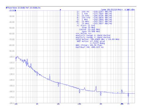
Figure 4: Typical phase-noise plot captured at the output of the SG7050EBN oscillator
