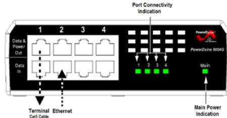
Figure 2: Connecting the PD-9004G
