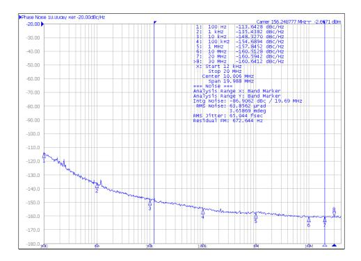
Figure 4: Typical phase-noise plot at the output of a VF901480 oscillator
