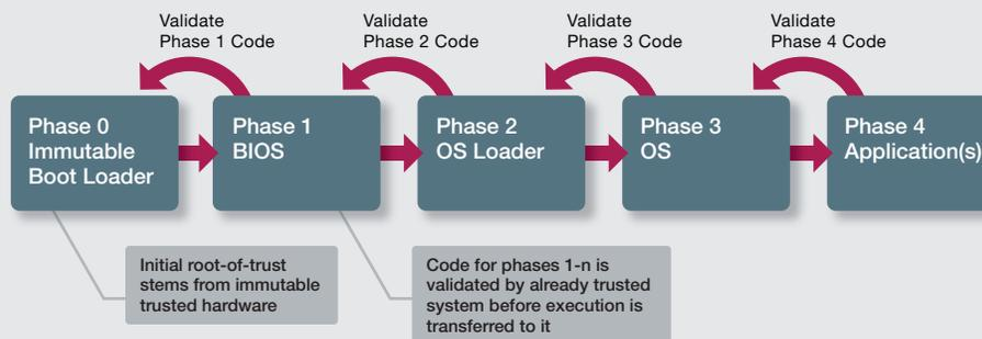
Secure boot starts from a trusted source and a process of authenticating each successive stage is performed to create a chain-of-trust as depicted in the above figure. With the Secure Boot reference design, trust can be extended to connected systems.
