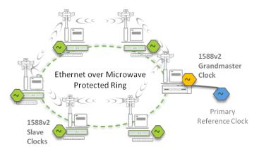
Fig. 5: Ring-based Backhaul Network with Grandmaster and Slave Clocking
