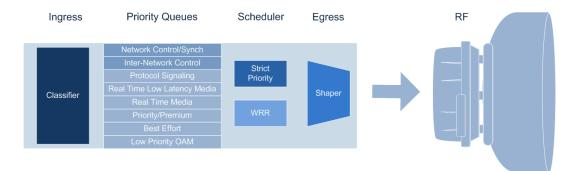
Fig. 3: Example of Microwave Traffic/QoS Management
