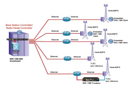
Fig. 1: IEEE-1588v2 Mobile Backhaul Implementation Example
