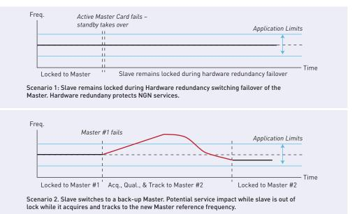
FIG. 3 IEEE 1588 PTP grandmaster clocks that employ hardware redundancy protect slave clocks from potential service impact during failover scenarios.
