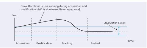
FIG. 2 Illustration of IEEE 1588 PTP slave clock acquisition and locking process. When the oscillator is locked, it can be held within the application limits for the target deployment requirements.
