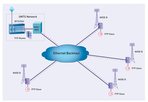
FIG. 1 Delivery of synchronization to next generation UMTS base stations will rely on PTP grandmaster clocks deployed in the MSC/RNC. Sync packets flow from the grandmaster clock to the slave clocks in the base stations.
