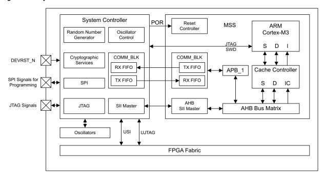
Figure 3, page 5 shows the system controller block in the IGLOO2 device. The architecture is similar to that in SmartFusion2, except that the COMM\_BLK in system controller communicates with COMM\_BLK in high performance memory subsystem (HPMS). A fabric master is required to use the NRBG services. Microsemi provides the CoreSysService Directcore IP with a simple user interface to use various NRBG system services.
