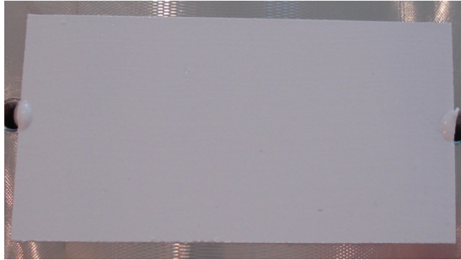
Picture 9: Grease on the heat sink before assembly
