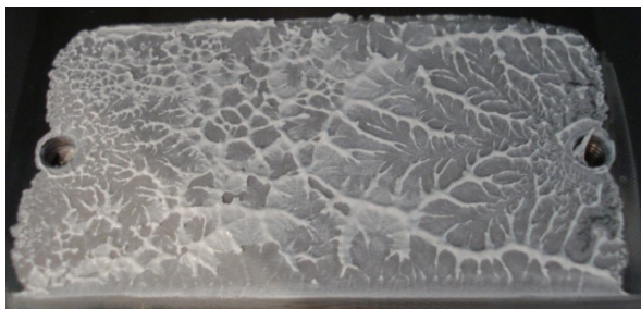
Picture 10: Grease on the heat sink after removing the module
