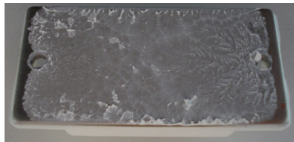
Picture 11: Grease on the module after disassembling
