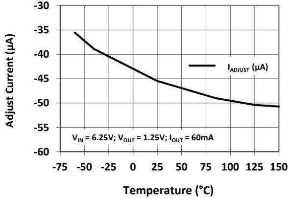
Figure 5 - Adjust Current vs. Temperature
