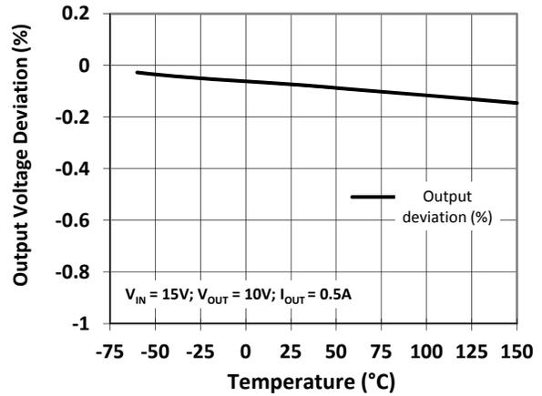
Figure 4 - Output Voltage Deviation vs. Temperature
