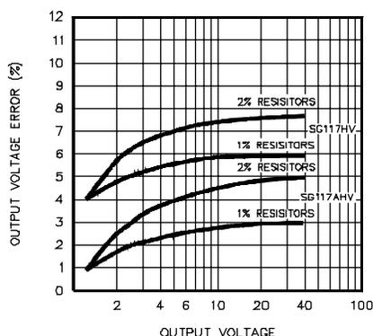
**Figure 14** - Voltage Tolerance vs. Resistor Tolerance
