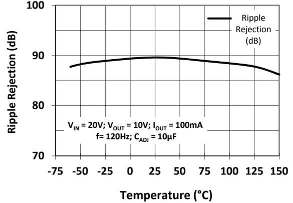
Figure 6 - Ripple Rejection vs. Temperature
