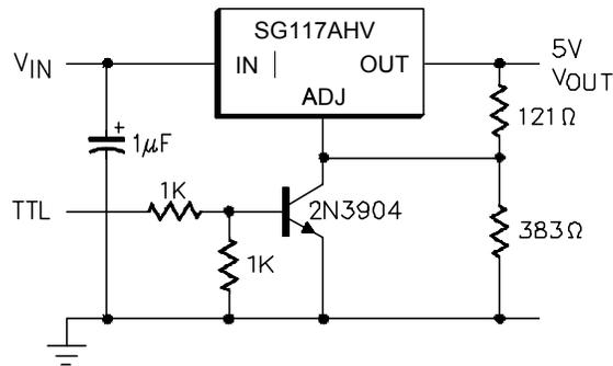
**Figure 19** - 5V Regulator with Shut Down
