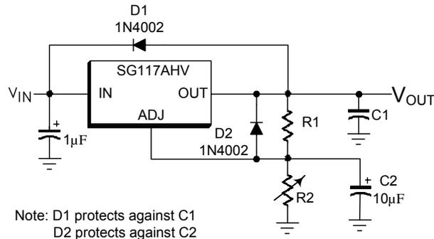
**Figure 16** - Use of Protection Diodes
