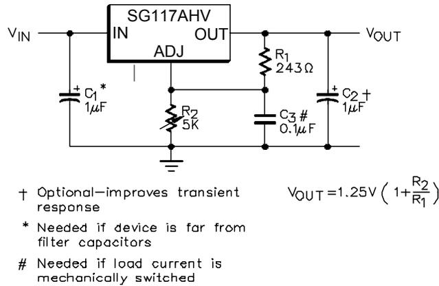
**Figure 18** - 1.2V – 25V Adjustable Regulator
