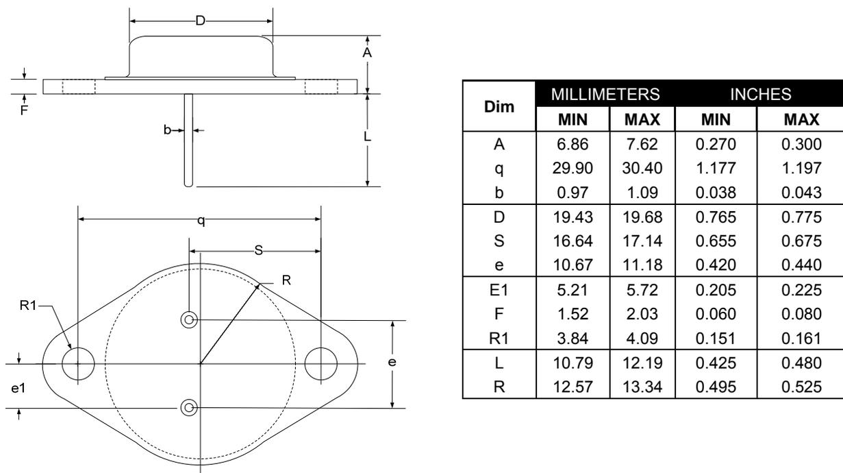
**Figure 25** - K 3-Pin TO-3 Package Dimensions
