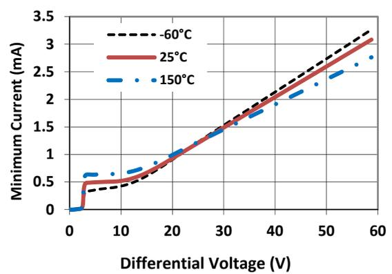
Figure 8 - Minimum Current vs. Input / Output Differential Voltage
