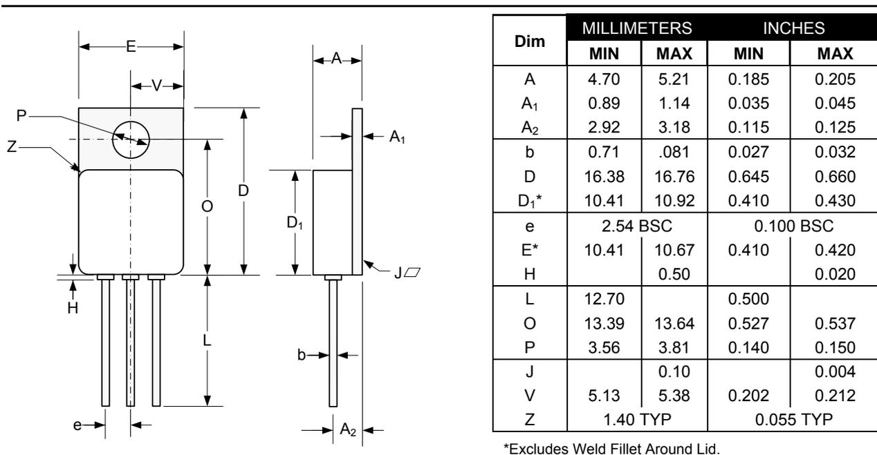
**Figure 24** - G/IG 3-Pin Hermetic TO-257 Package Dimensions
