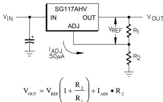
**Figure 13** - Basic Regulator Circuit
