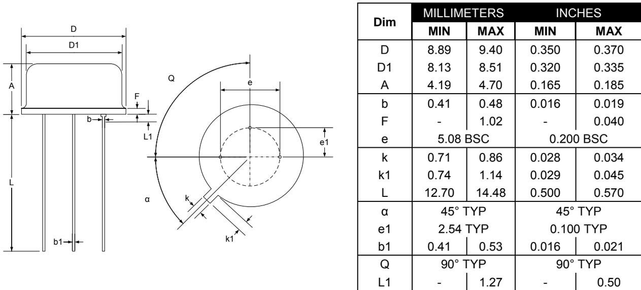
Figure 22 • T 3-Pin Metal Can TO-39 Package Dimensions
