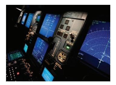
With the introduction of the fly-by-wire (FBW) electronic flight control avionics system, the movement of flight controls are converted to electronic signals transmitted by wires and the flight control computers determine how to move the actuators at each control surface to provide the expected response.
