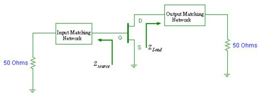
Note:  $Z_{\text{source}}$  is looking into the input circuit;  $Z_{Load}$  is looking into the output circuit.
