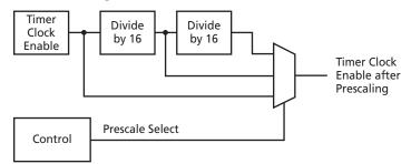
Figure 9-3. Prescale Clock Enable Generation
