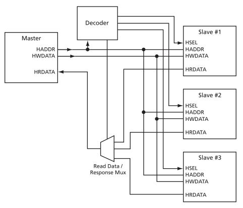
Figure 2-1. AHB-Lite Block Diagram
