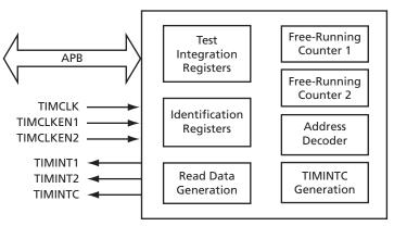
Figure 9-1. Dual Input Timer Block Diagram
