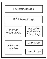
Figure 7-1. Interrupt Controller Block Diagram
