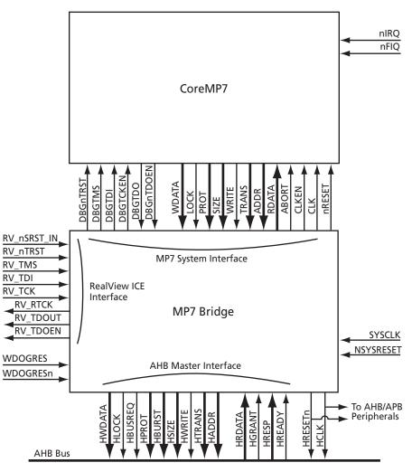
Figure 1-1. CoreMP7 and MP7Bridge Connections
