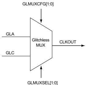
The signal assigned to the GCAx pins (Example: GCA0/IO36NDB1V0, GCA1/IO36PDB1V0, and others) as a CLKBUF or CLKBUF\_LVPECL or CLKBUF\_LVDS goes through the glitchless mux. For the glitchless mux to operate correctly, the signal must be a free-running clock signal. See the "**Glitchless MUX**" section in the *SmartFusion Microcontroller Subsystem User Guide* for more information. Verify that the signal driving this instance is a continuous clock signal.
