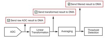
In Libero SoC v10 SP1, the PPE microcode is incorrectly generated when **Send filtered value to DMA** is enabled. Prior to Libero SoC v10 SP1 the microcode was generated correctly.
