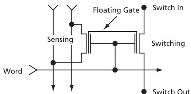
**Figure 3: ProASIC3/E Flash-Based Switch**
