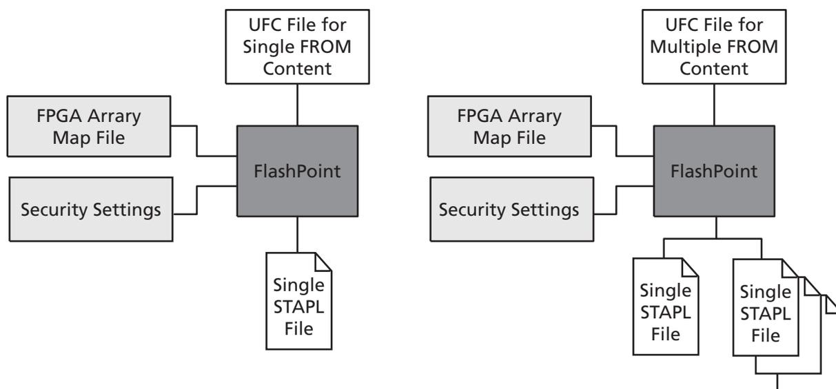
Figure 10: Generation of Programming Files Using FlashPoint
