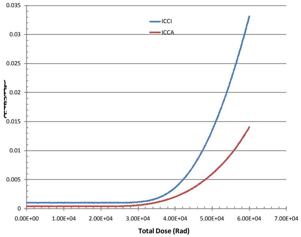
Figure 5 DUT 203 in-flux  $I_{CCA}$  and  $I_{CCI}$
