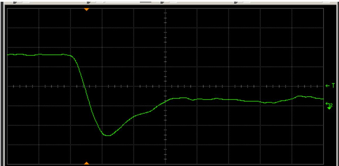
Figure 18(b) DUT 225 post-annealing falling edge. The ordinate is 2 V/div, and abscissa 2 ns/div.
