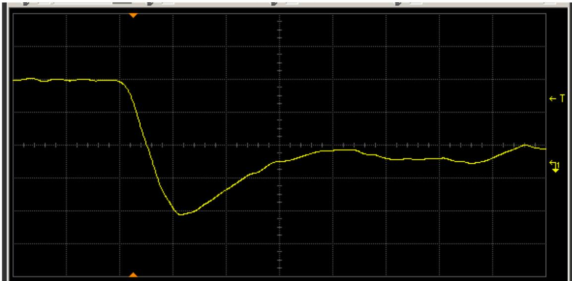
Figure 19(a) DUT 236 pre-irradiation falling edge. The ordinate is 2 V/div, and abscissa 2 ns/div.
