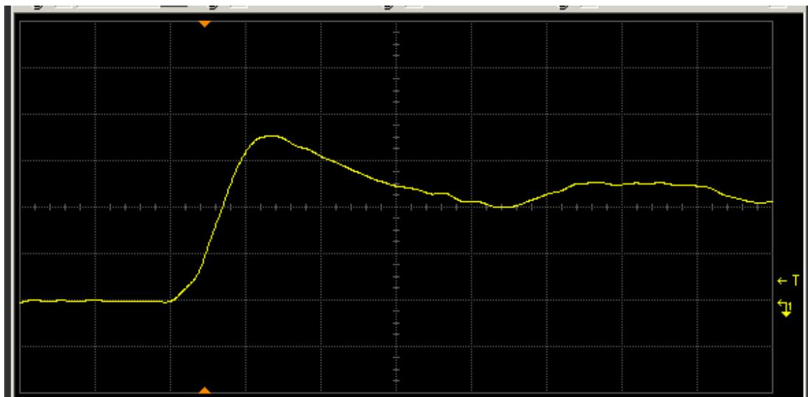
Figure 10(a) DUT 107 pre-radiation rising edge. The ordinate is 2 V/div, and abscissa 2 ns/div.
