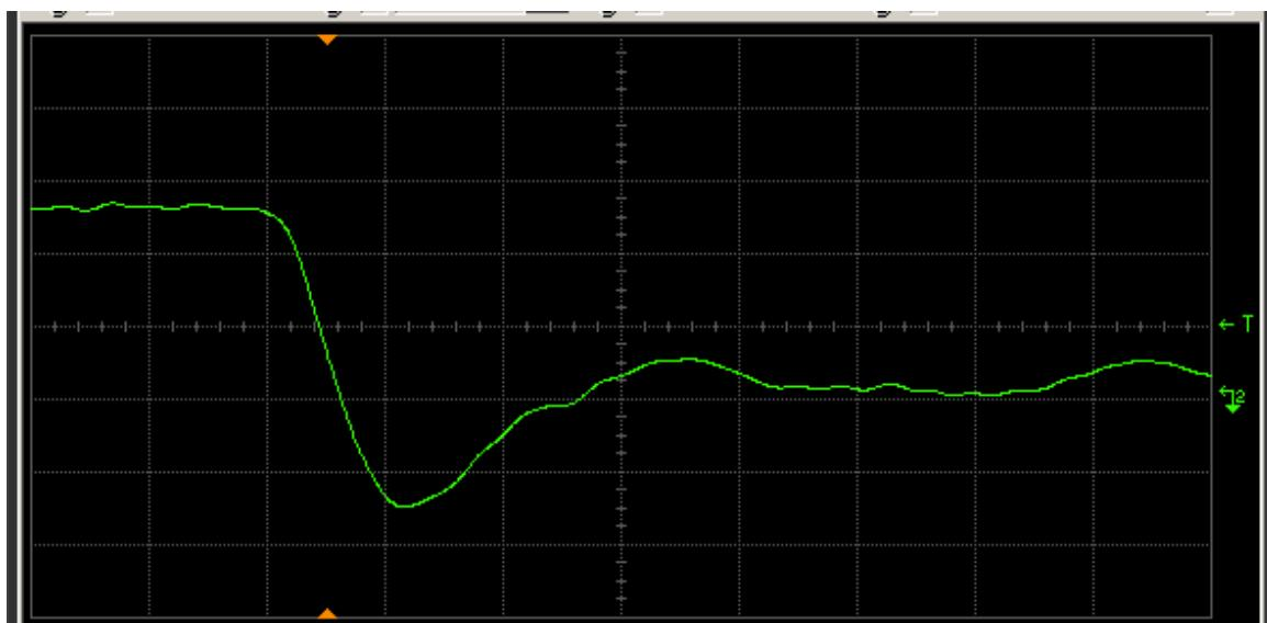
Figure 16(b) DUT 107 post-annealing falling edge. The ordinate is 2 V/div, and abscissa 2 ns/div.
