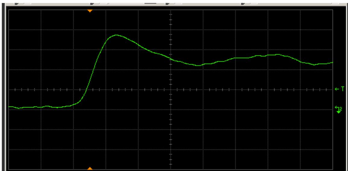
Figure 10(b) DUT 107 post-annealing rising edge. The ordinate is 2 V/div, and abscissa 2 ns/div.
