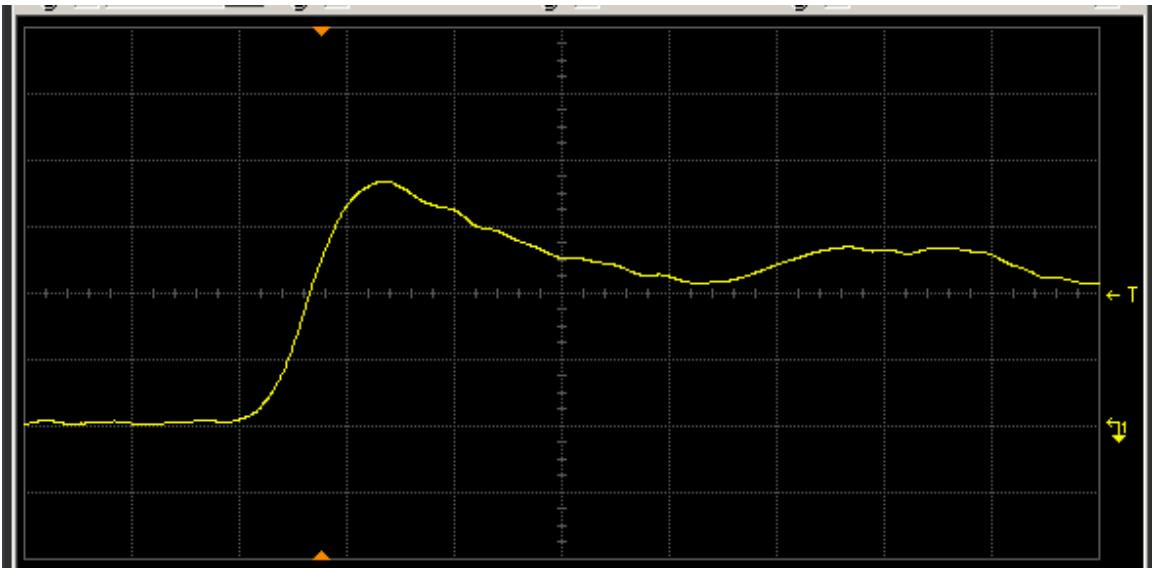
Figure 12(a) DUT 225 pre-irradiation rising edge. The ordinate is 2 V/div, and abscissa 2 ns/div.
