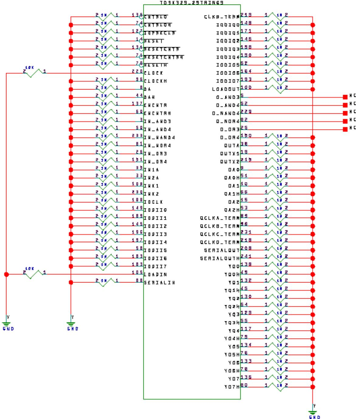
Figure A1 DUT bias during irradiation
