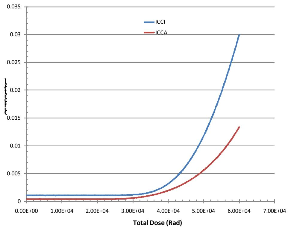
Figure 7 DUT 236 in-flux  $I_{CCA}$  and  $I_{CCI}$
