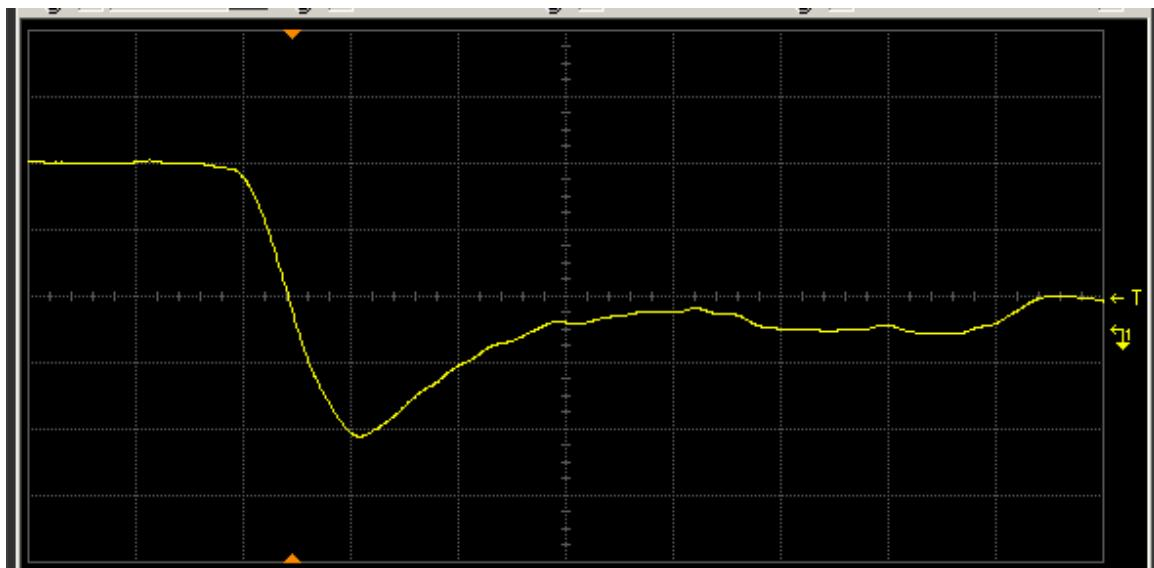
Figure 15(a) DUT 77 pre-irradiation falling edge. The ordinate is 2 V/div, and abscissa 2 ns/div.
