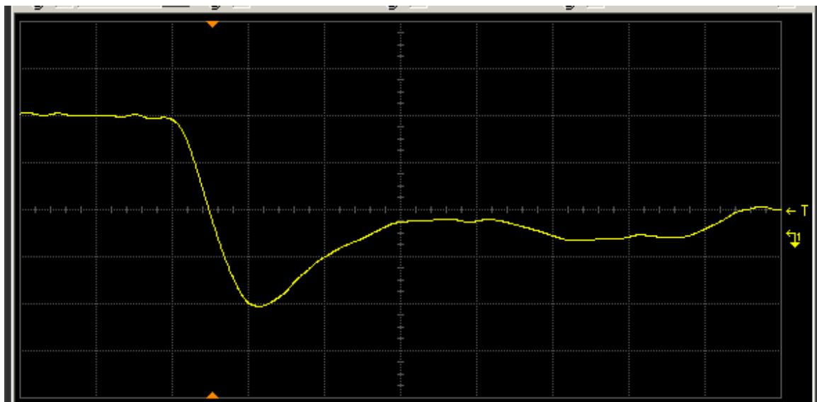
Figure 16(a) DUT 107 pre-radiation falling edge. The ordinate is 2 V/div, and abscissa 2 ns/div.
