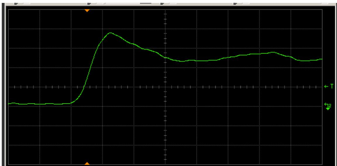
Figure 11(b) DUT 203 post-annealing rising edge. The ordinate is 2 V/div, and abscissa 2 ns/div.
