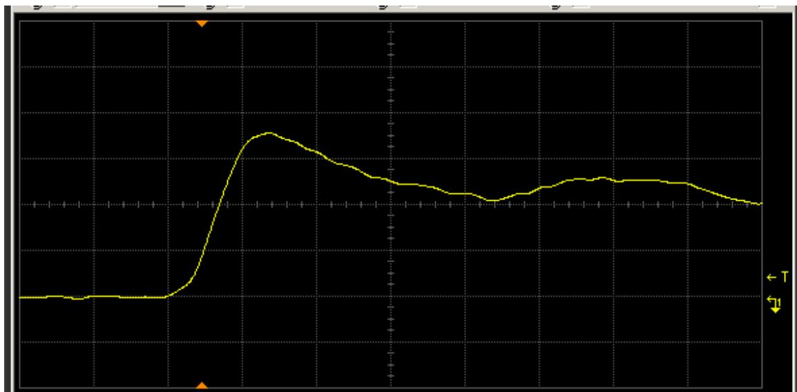
Figure 9(a) DUT 77 pre-irradiation rising edge. The ordinate is 2 V/div, and abscissa 2 ns/div.
