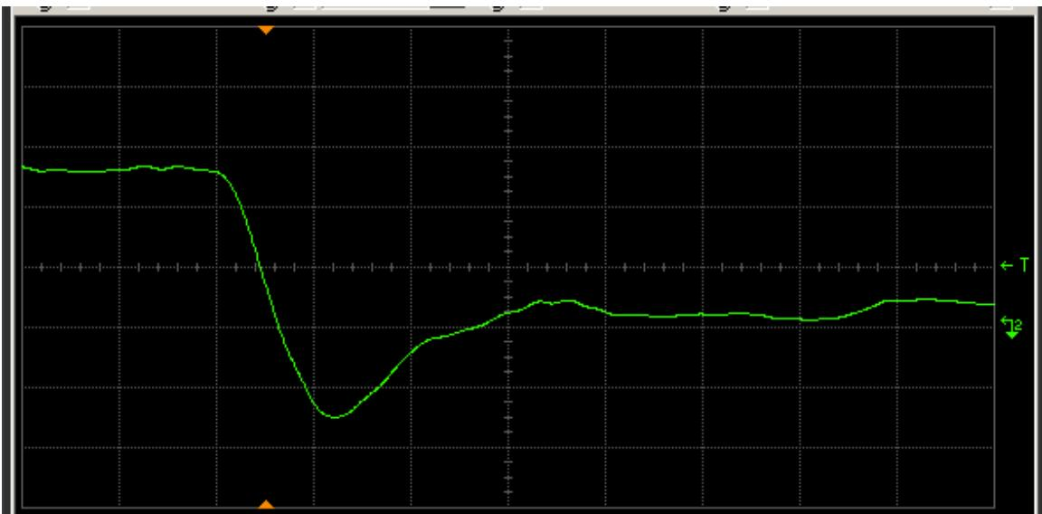
Figure 14(b) DUT 25 post-annealing falling edge. The ordinate is 2 V/div, and abscissa 2 ns/div.
