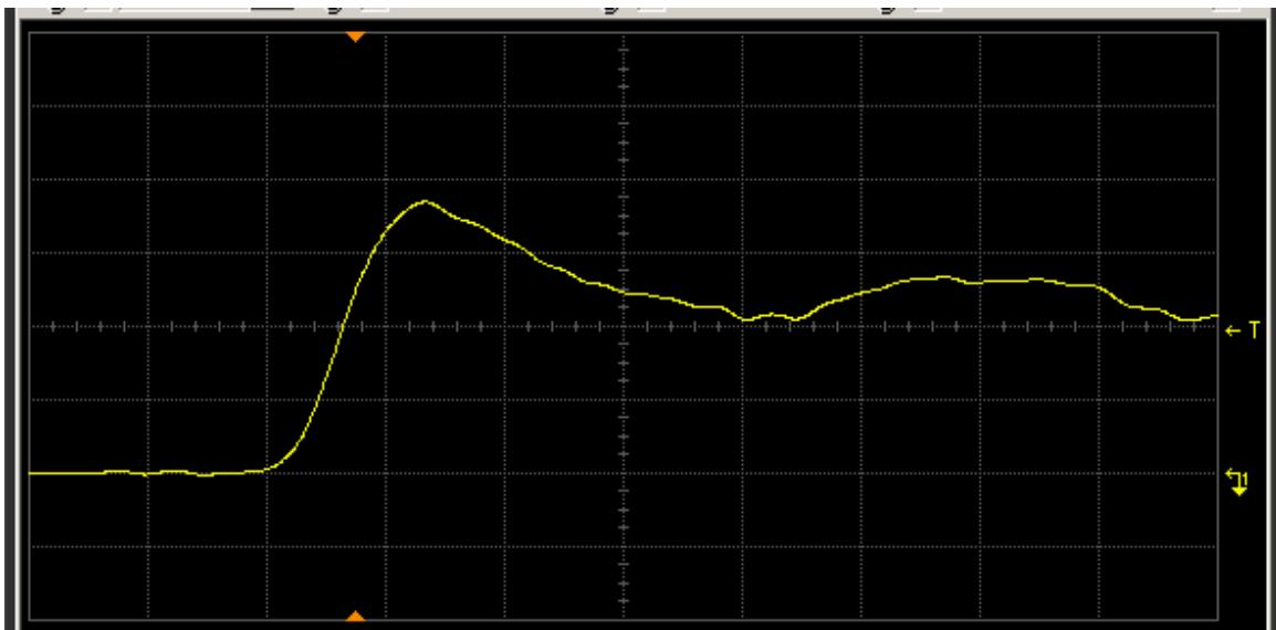
Figure 13(a) DUT 236 pre-irradiation rising edge. The ordinate is 2 V/div, and abscissa 2 ns/div.
