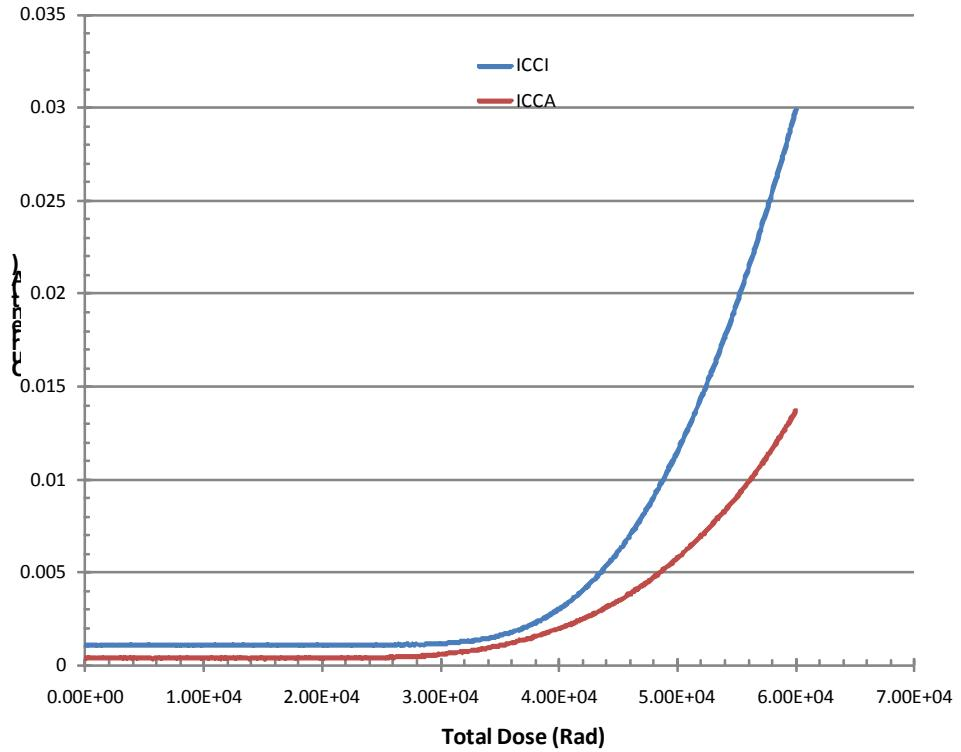
Figure 6 DUT 225 in-flux  $I_{CCA}$  and  $I_{CCI}$
