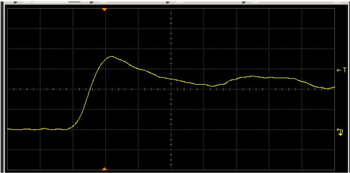
Figure 8(a) DUT 25 pre-irradiation rising edge. The ordinate is 2 V/div, and abscissa 2 ns/div.
