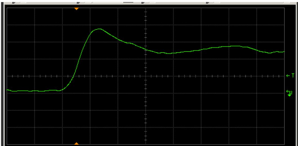
Figure 13(b) DUT 236 post-annealing rising edge. The ordinate is 2 V/div, and abscissa 2 ns/div.
