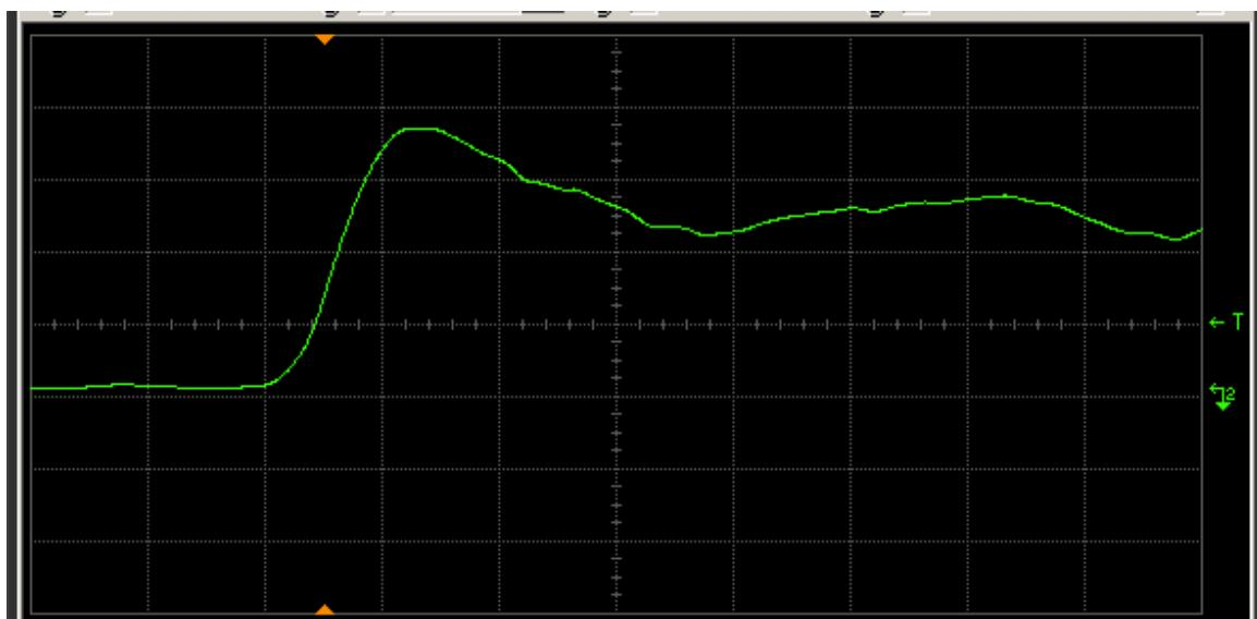
Figure 9(b) DUT 77 post-annealing rising edge. The ordinate is 2 V/div, and abscissa 2 ns/div.
