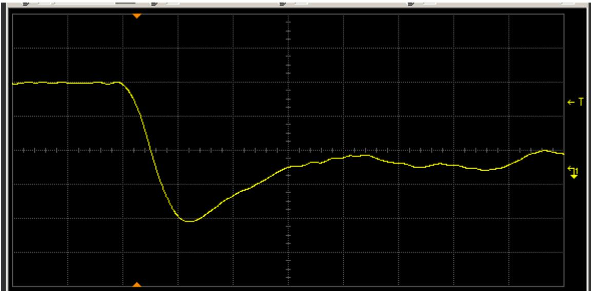
Figure 18(a) DUT 225 pre-irradiation falling edge. The ordinate is 2 V/div, and abscissa 2 ns/div.
