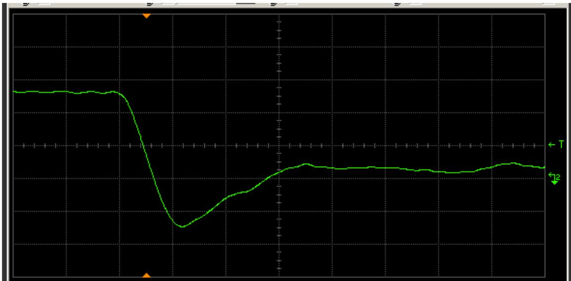
Figure 19(b) DUT 236 post-annealing falling edge. The ordinate is 2 V/div, and abscissa 2 ns/div.
