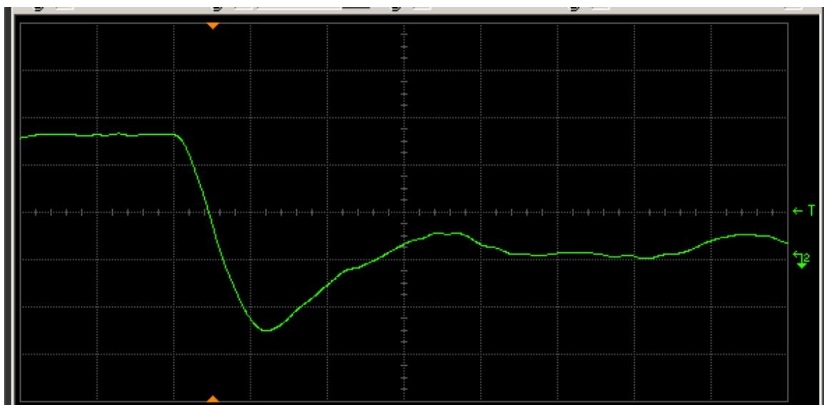
Figure 15(b) DUT 77 post-annealing falling edge. The ordinate is 2 V/div, and abscissa 2 ns/div.
