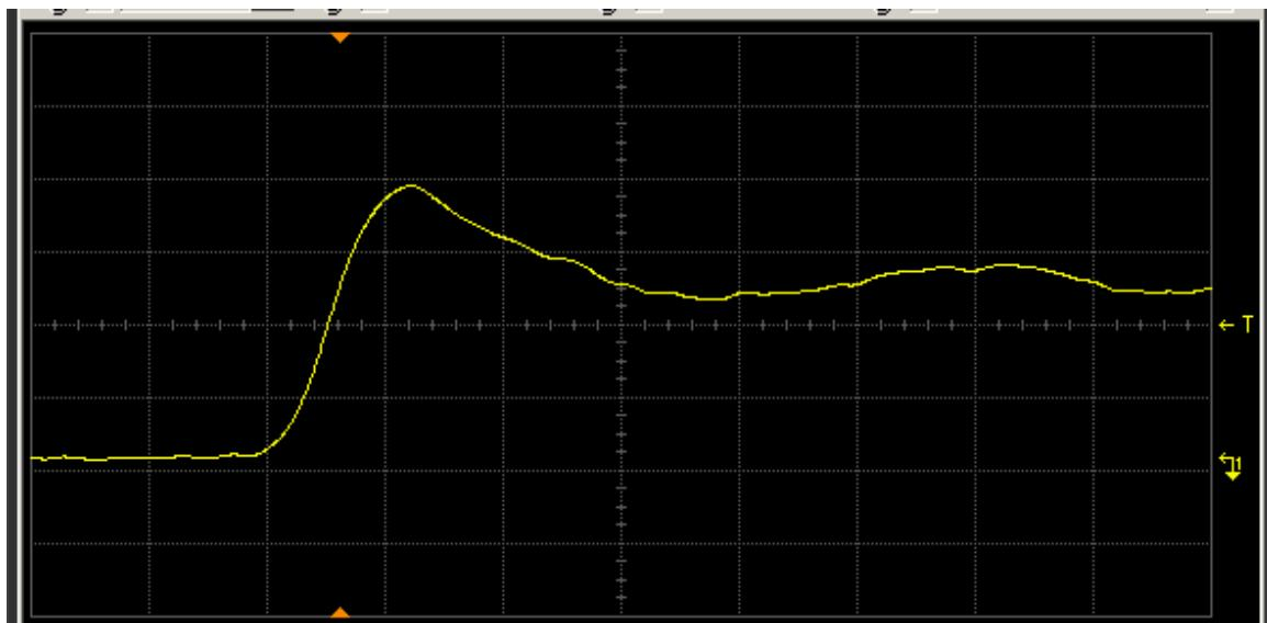
Figure 11(a) DUT 203 pre-irradiation rising edge. The ordinate is 2 V/div, and abscissa 2 ns/div.
