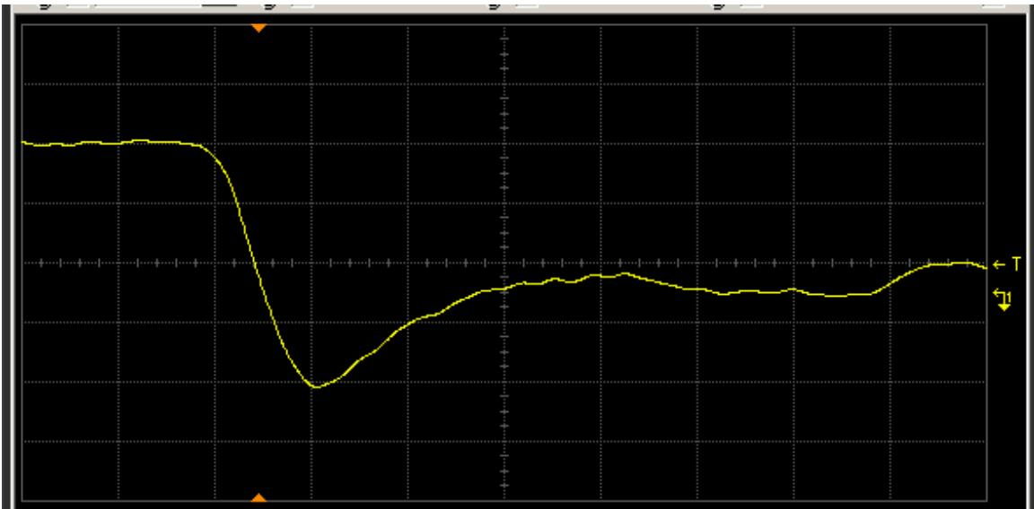
Figure 14(a) DUT 25 pre-irradiation falling edge. The ordinate is 2 V/div, and abscissa 2 ns/div.
