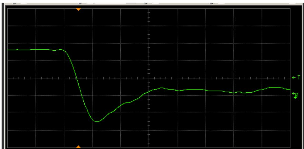
Figure 17(b) DUT 203 post-annealing falling edge. The ordinate is 2 V/div, and abscissa 2 ns/div.
