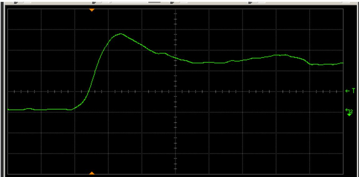
Figure 8(b) DUT 25 post-annealing rising edge. The ordinate is 2 V/div, and abscissa 2 ns/div.
