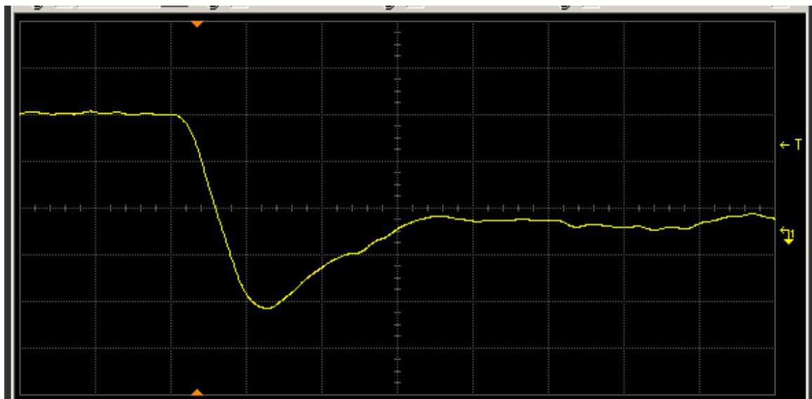
Figure 17(a) DUT 203 pre-irradiation falling edge. The ordinate is 2 V/div, and abscissa 2 ns/div.
