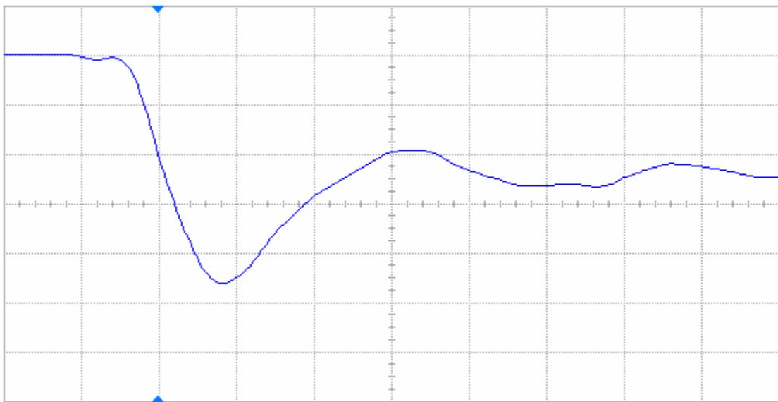
Figure 10(b) DUT 81978 post-annealing falling edge, abscissa scale is 2 V/div and ordinate scale is 2 ns/div.
