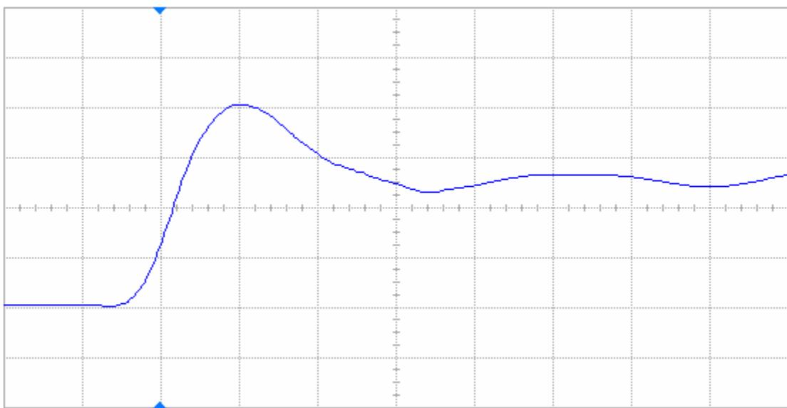
Figure 8(b) DUT 82050 post-annealing rising edge, abscissa scale is 2 V/div and ordinate scale is 2 ns/div.
