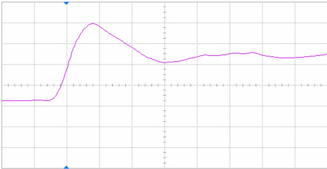
Figure 8(a) DUT 82050 pre-irradiation rising edge, abscissa scale is 2 V/div and ordinate scale is 2 ns/div.
