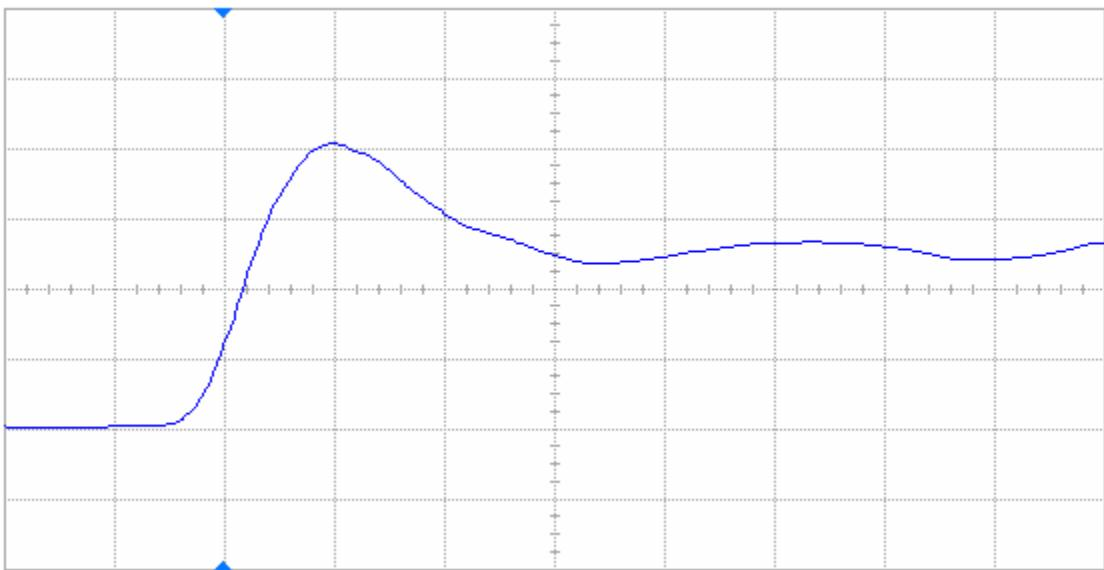
Figure 9(b) DUT 82133 post-annealing rising edge, abscissa scale is 2 V/div and ordinate scale is 2 ns/div.
