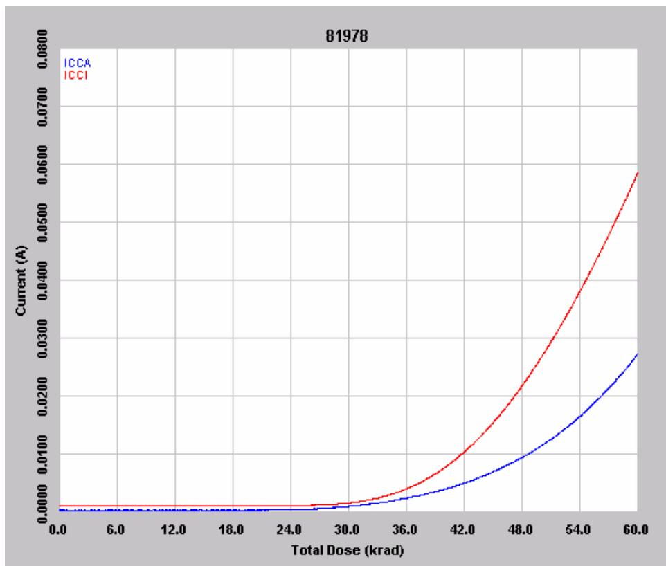
Figure 2 In flux  $I_{CCA}$  and  $I_{CCI}$  of DUT 81978, 60 krad total dose
