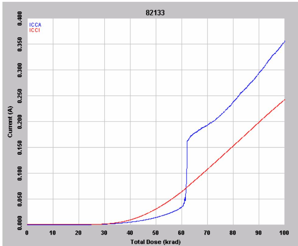
Figure 5 In flux  $I_{CCA}$  and  $I_{CCI}$  of DUT 82133, 100 krad total dose
