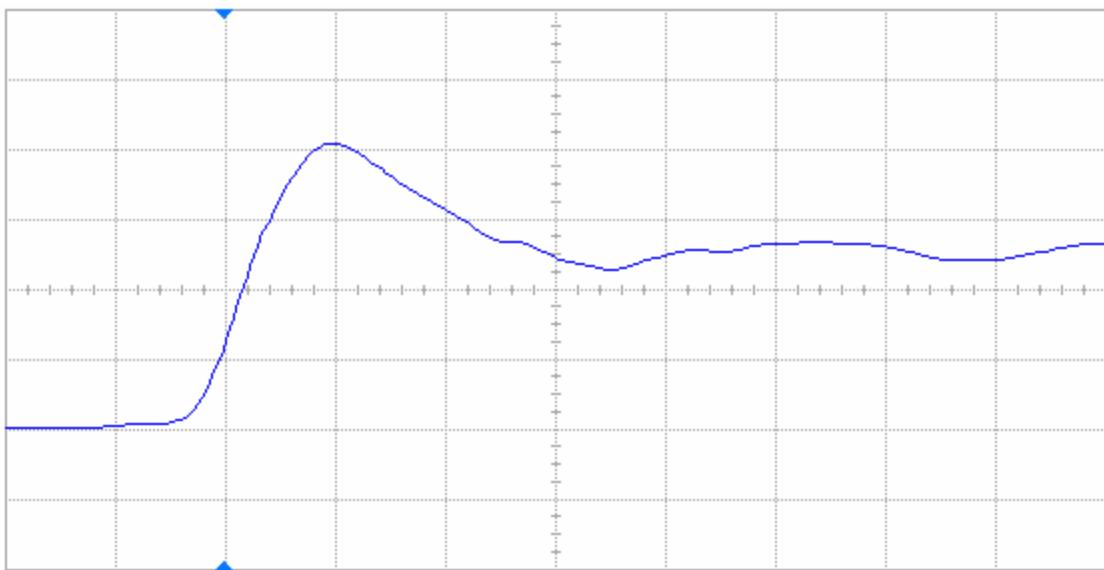
Figure 7(b) DUT 82036 post-annealing rising edge, abscissa scale is 2 V/div and ordinate scale is 2 ns/div.
