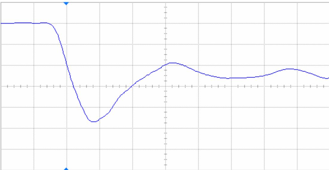
Figure 13(b) DUT 82133 post-irradiation falling edge, abscissa scale is 2 V/div and ordinate scale is 2 ns/div.
