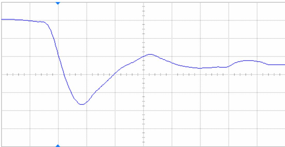
Figure 11(b) DUT 82036 post-annealing falling edge, abscissa scale is 2 V/div and ordinate scale is 2 ns/div.
