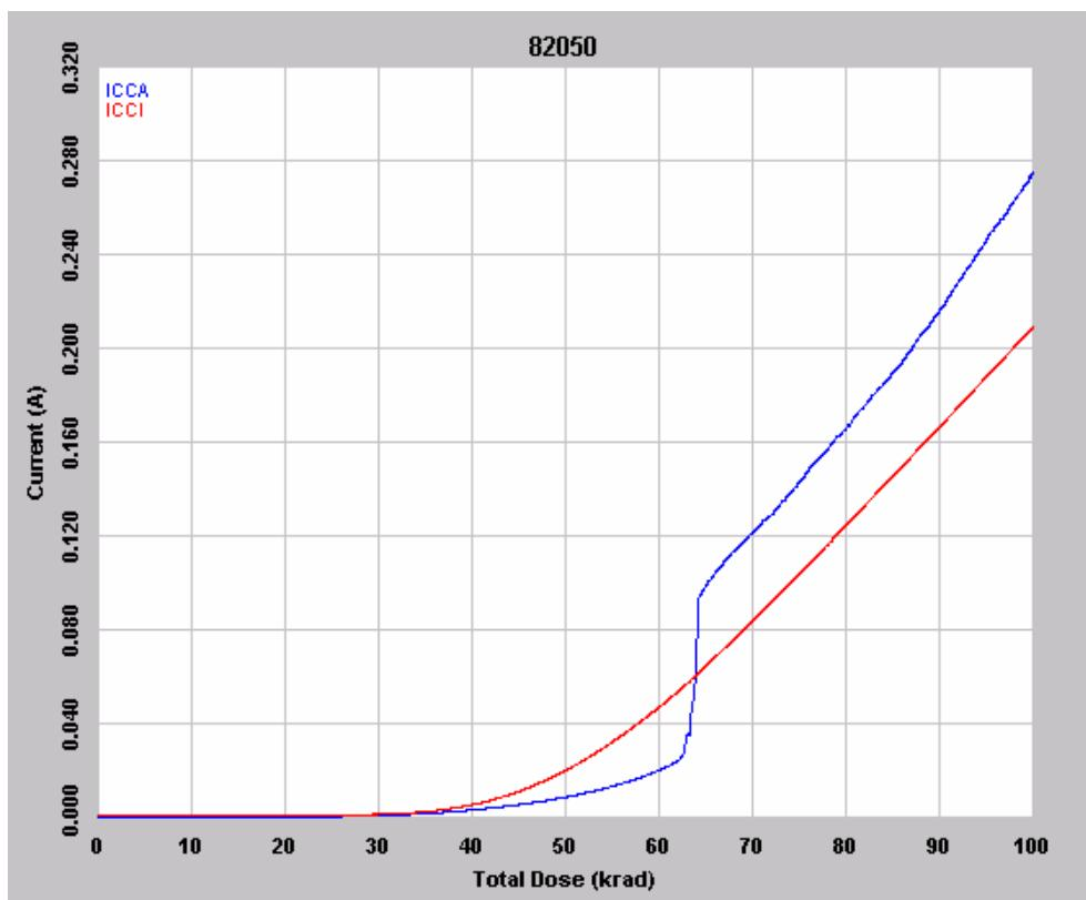
Figure 4 In flux  $I_{CCA}$  and  $I_{CCI}$  of DUT 82050, 100 krad total dose
