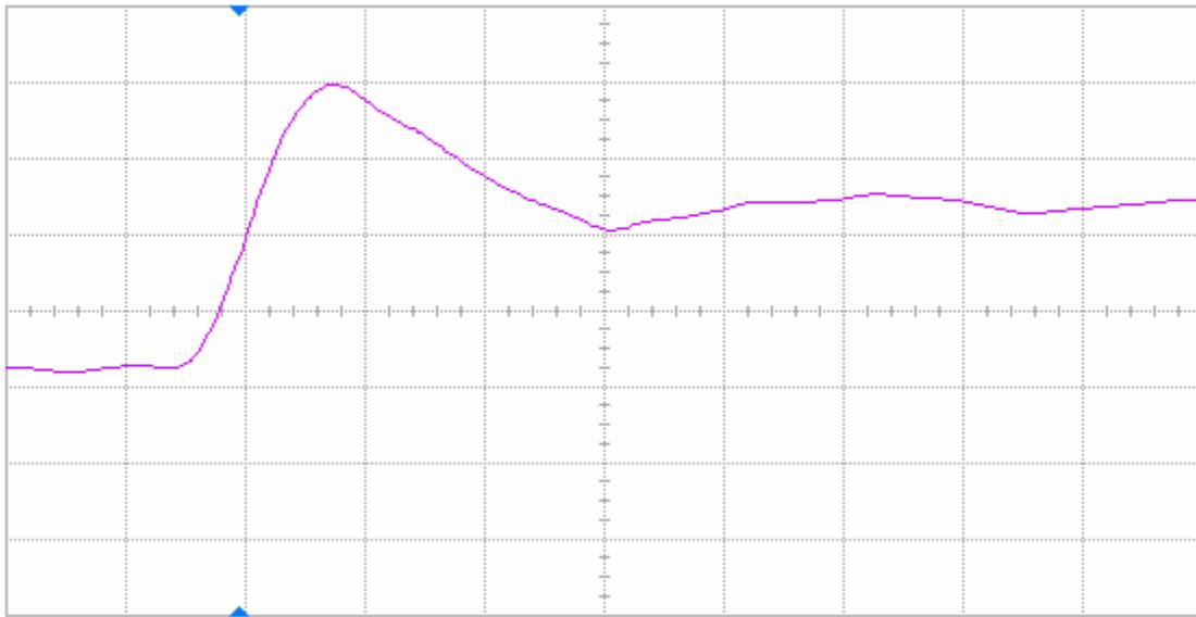
Figure 6(a) DUT 81978 pre-irradiation rising edge, abscissa scale is 2 V/div and ordinate scale is 2 ns/div.
