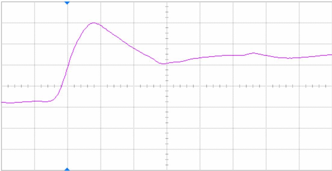
Figure 9(a) DUT 82133 pre-irradiation rising edge, abscissa scale is 2 V/div and ordinate scale is 2 ns/div.
