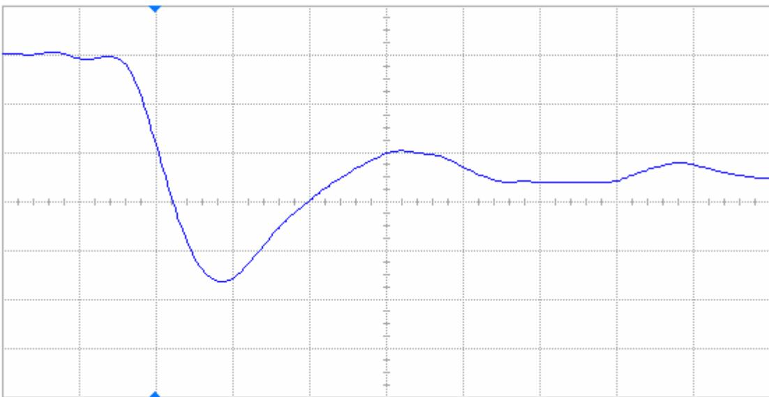
Figure 12(b) DUT 82050 post-annealing falling edge, abscissa scale is 2 V/div and ordinate scale is 2 ns/div.
