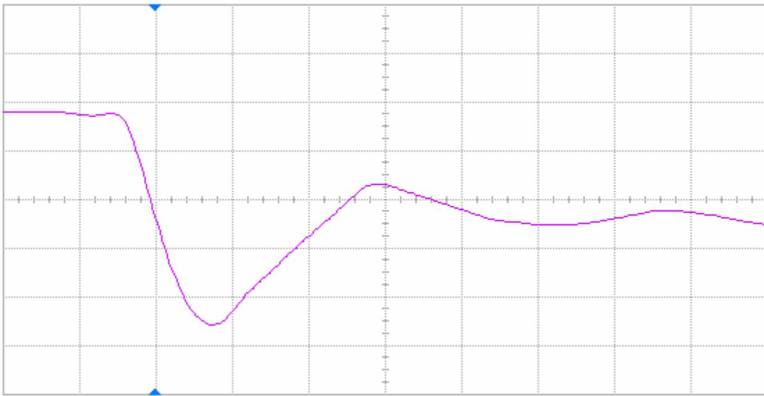
Figure 13(a) DUT 82133 pre-irradiation falling edge, abscissa scale is 2 V/div and ordinate scale is 2 ns/div.
