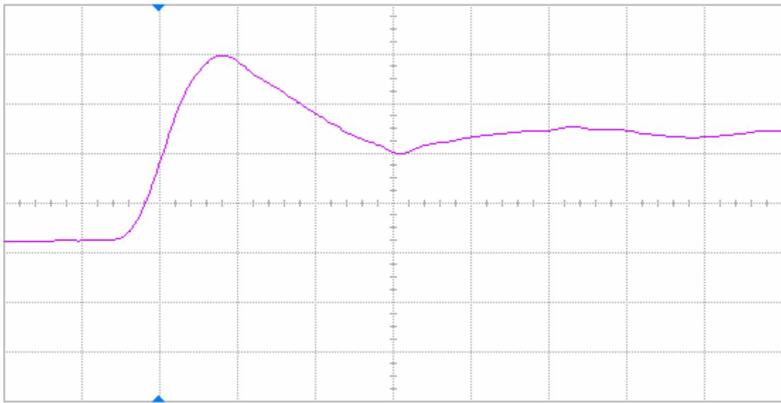
Figure 7(a) DUT 82036 pre-irradiation rising edge, abscissa scale is 2 V/div and ordinate scale is 2 ns/div.
