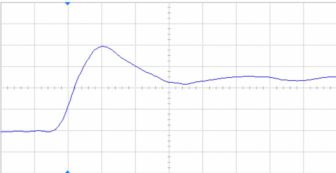
Figure 6(b) DUT 81978 post-annealing rising edge, abscissa scale is 2 V/div and ordinate scale is 2 ns/div.
