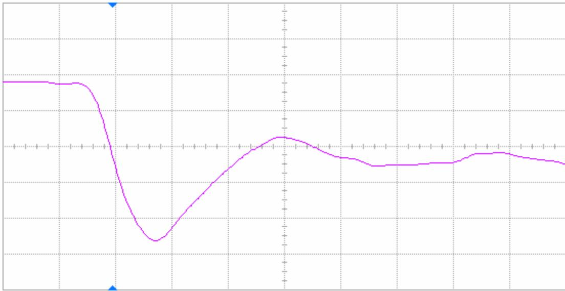
Figure 10(a) DUT 81978 pre-irradiation falling edge, abscissa scale is 2 V/div and ordinate scale is 2 ns/div.
