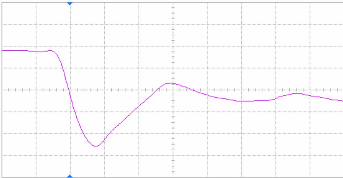
Figure 11(a) DUT 82036 pre-irradiation falling edge, abscissa scale is 2 V/div and ordinate scale is 2 ns/div.
