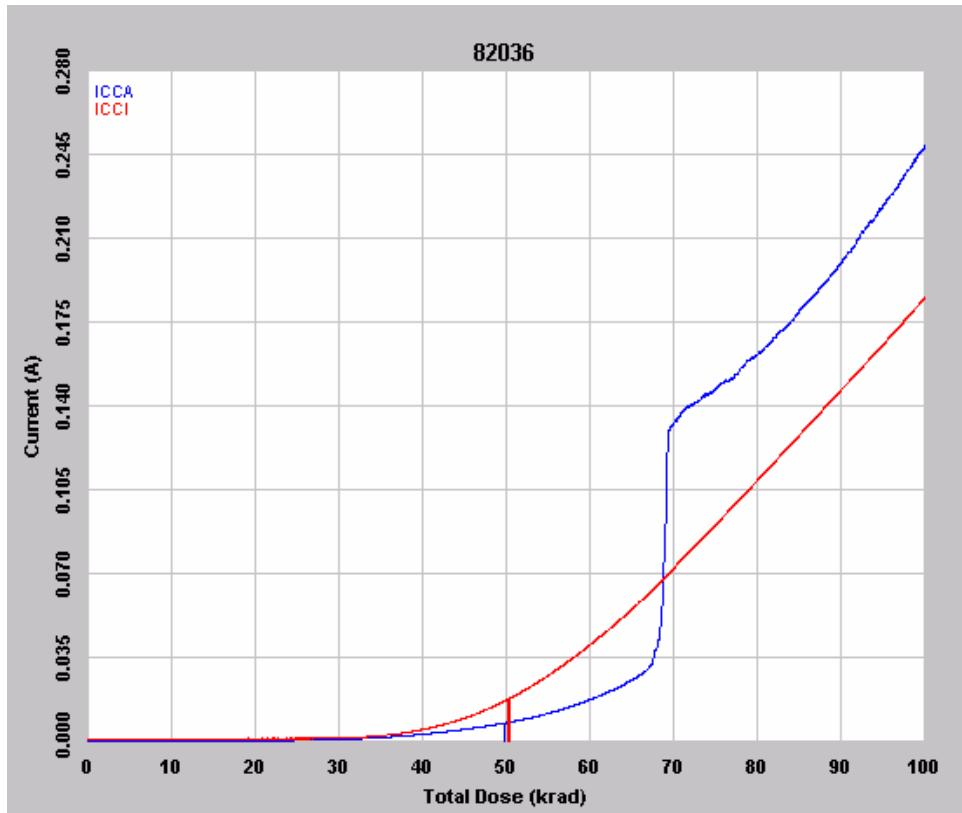
Figure 3 In flux  $I_{CCA}$  and  $I_{CCI}$  of DUT 82036, 100 krad total dose
