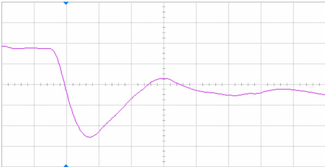
Figure 12(a) DUT 82050 pre-irradiation falling edge, abscissa scale is 2 V/div and ordinate scale is 2 ns/div.
