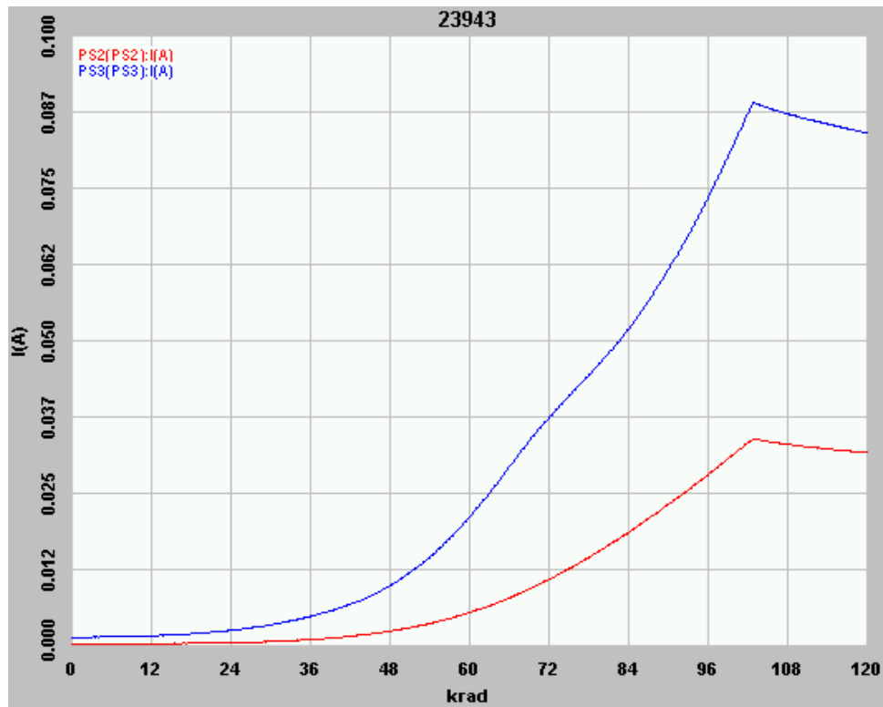
Figure5 In-flux I_{CC} of DUT 23943, PS2 supplies I_{CCI} and PS3 supplies I_{CCA} .
