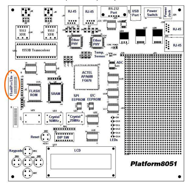
6. Connect the FlashPro Lite to the PC's parallel port.
