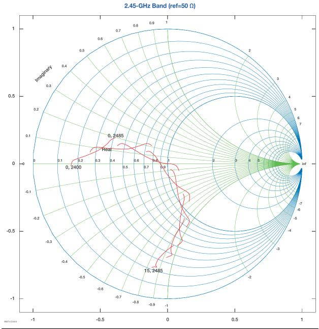
Figure 2-2 • Combined Port Impedance (2400 to 2485GHz)
