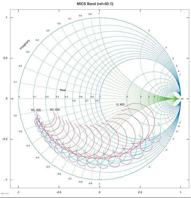
Figure 2-1 • Combined Port Impedance (402 to 405 MHz)
