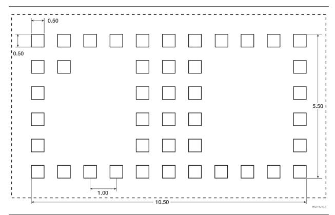
Figure 4-3 • Recommended PCB Layout
