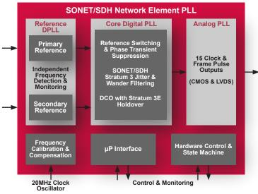
The ZL<sup>™</sup> 30407 is a digital phase locked loop (DPLL) that synchronizes SONET (Synchronous Optical Network) and SDH (Synchronous Digital Hierarchy) network equipment.
