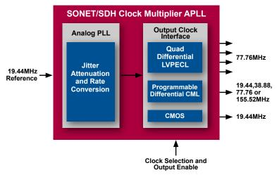
The ZL™30406 is the world's first SONET (synchronous optical network) and SDH (synchronous digital hierarchy) clock multiplier analog phase locked loop (APLL) to provide six output clocks from a single device with jitter performance that surpasses OC-48 and STM-16 system requirements. This unique level of integration and performance allows designers of SONET and SDH networking equipment to meet stringent timing requirements.
