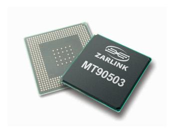
The MT90503 is a multi-channel ATM Adaptation Layer 1 (AAL1) segmentation and reassembly (SAR) device that interfaces serial stream voice and data traffic from the TDM bus to the ATM network. The device provides the industry's highest integration—SONET 155Mbps or SDH OC3 bandwidth in a single-chip—substantially reducing cost, board space and power consumption compared to alternative solutions.
