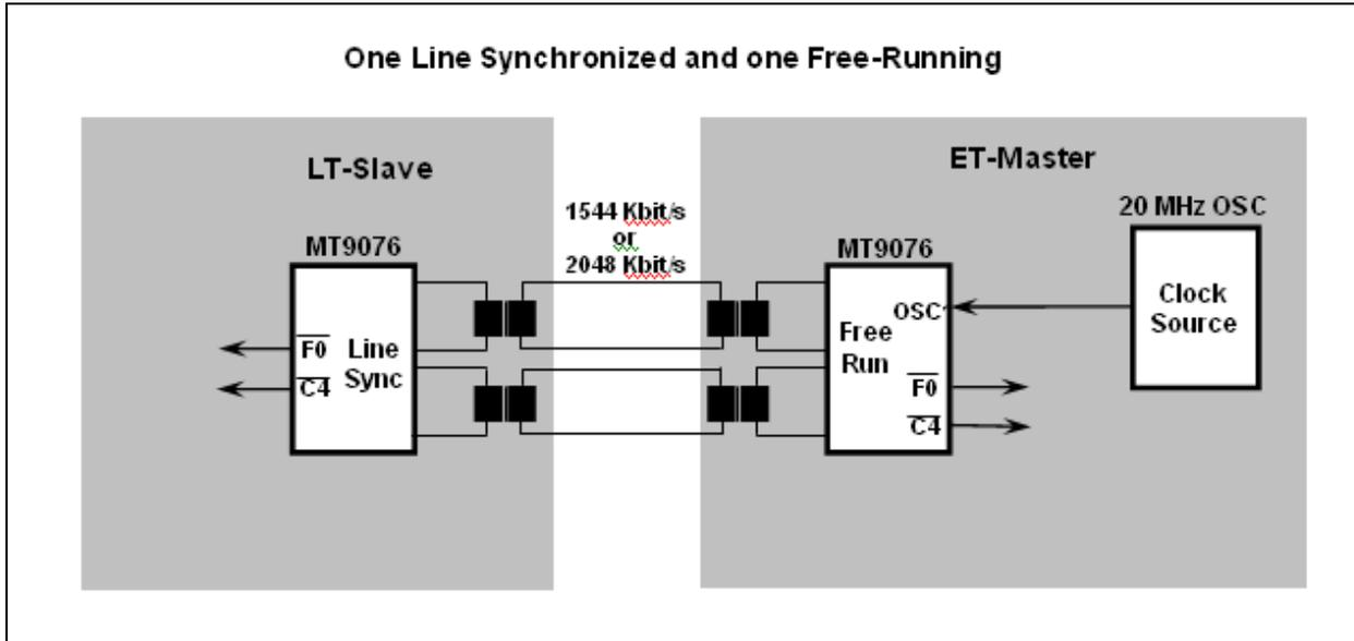
Figure 1 - Point to Point Master Slave Timing Configuration
