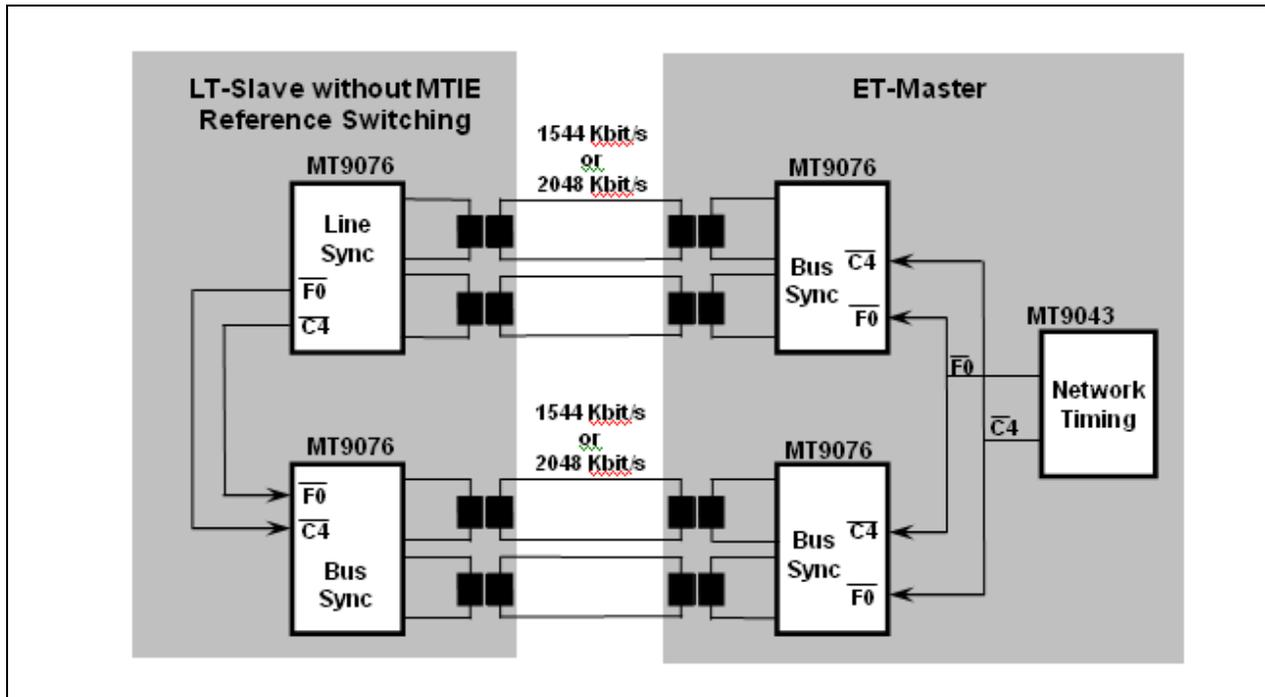
Figure 2 - Allows use of one PLL, but the timing will not be as robust as synchronization will be lost if the line in the slave link cards between two framers is broken.
