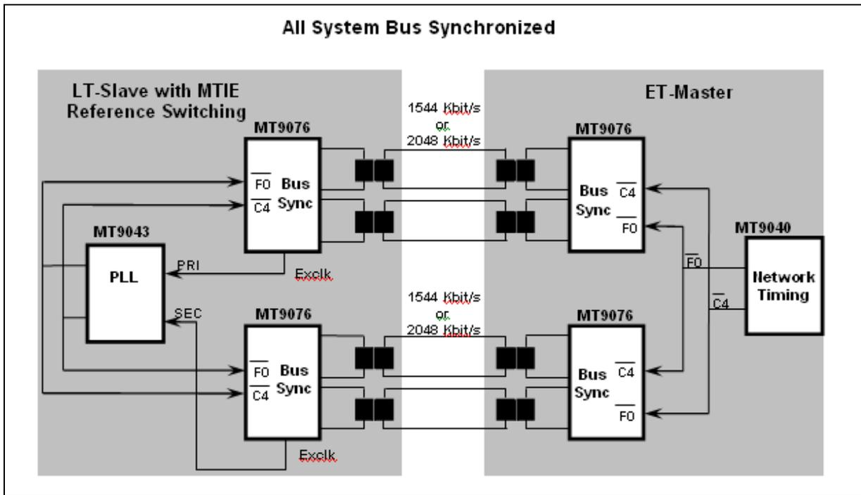
Figure 3 - A more resilient configuration, regarding an extra PLL with two reference inputs. The extracted clock is supplied to the MT9043 PLL which generates the synchronized timing for the system
