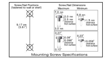
2. Align the PD-9501G mounting slots to capture the surface screws
