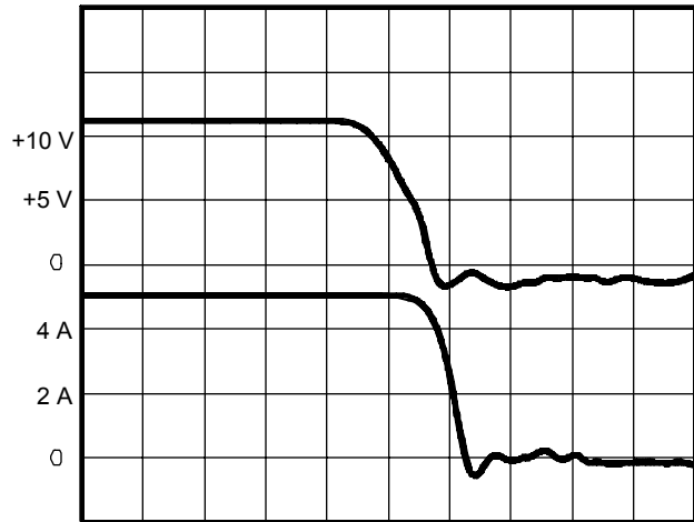
Figure 17. MOSFETS Turn-Off Waveforms. Upper Trace: Gate Voltage @ 100 ns/div. Lower Trace: Drain Current @ 100 ns/div.
