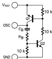
3. Another way of providing greater deadband is just to limit the maximum pulse width. This can be done by using a clamp to limit the output voltage of the error amplifier. A simple way of achieving this clamp is with the circuit below:
