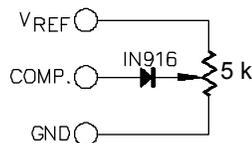
This circuit will limit the error amplifier's voltage range since its current source output will supply only 100  $\mu$ A. Another advantage of this circuit is that it does not change the programmed oscillator frequency.
