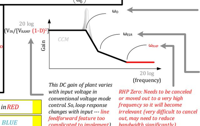
**Figure 5:** Plant Transfer Function for a Buck-Boost, Using VMC
