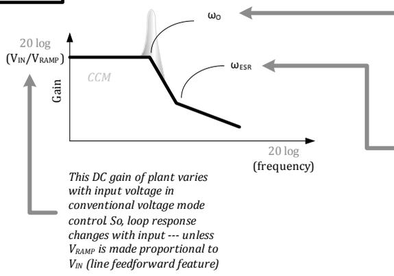
The double LC pole occurs here. There can be severe peaking in the gain plot right here, because of high Quality factor [ $Q=Rv(C/L)$ ]. This is also accompanied by a sudden 180 degrees phase shift that can lead to instability or (ringing).
