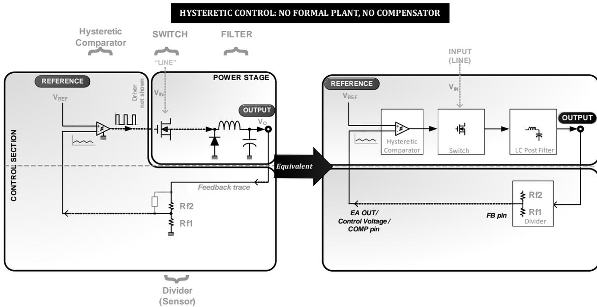
**Figure 10:** Functional Blocks of the Hysteretic Converter
