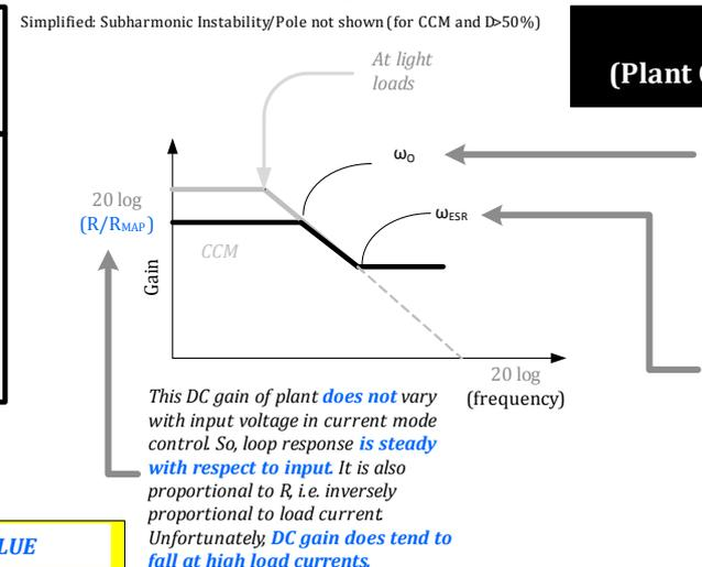
**Figure 6:** Plant Transfer Function for a Buck, Using CMC
