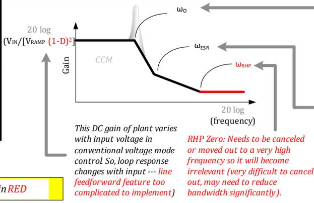
The double LC pole occurs here. There can be severe peaking in the gain plot right here, because of high Quality factor [ $Q=Rv(C/L)$ ]. This is also accompanied by a sudden 180 degrees phase shift that can lead to instability or (ringing).
