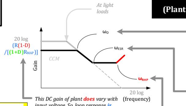
Output "load pole". **Single pole, no peaking.** Its location is inversely proportional to R, so it is proportional to load current. DC gain is inversely proportional to load current. So crossover frequency (bandwidth) is unchanged as load changes (dashed line)
