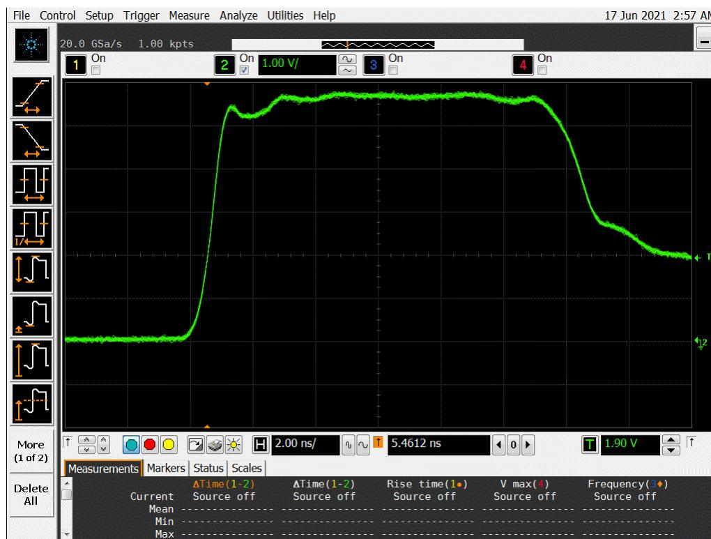
**Figure 13a DUT 2326 Pre-Irradiation Rising Edge**
