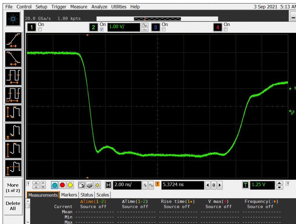
**Figure 17b DUT 2338 Post-Annealing Falling Edge**
