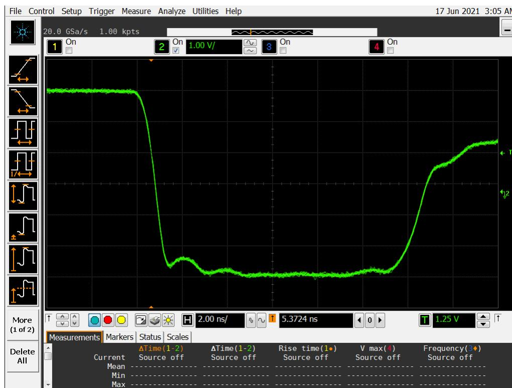
**Figure 15a DUT 2352 Pre-Radiation Falling Edge**
