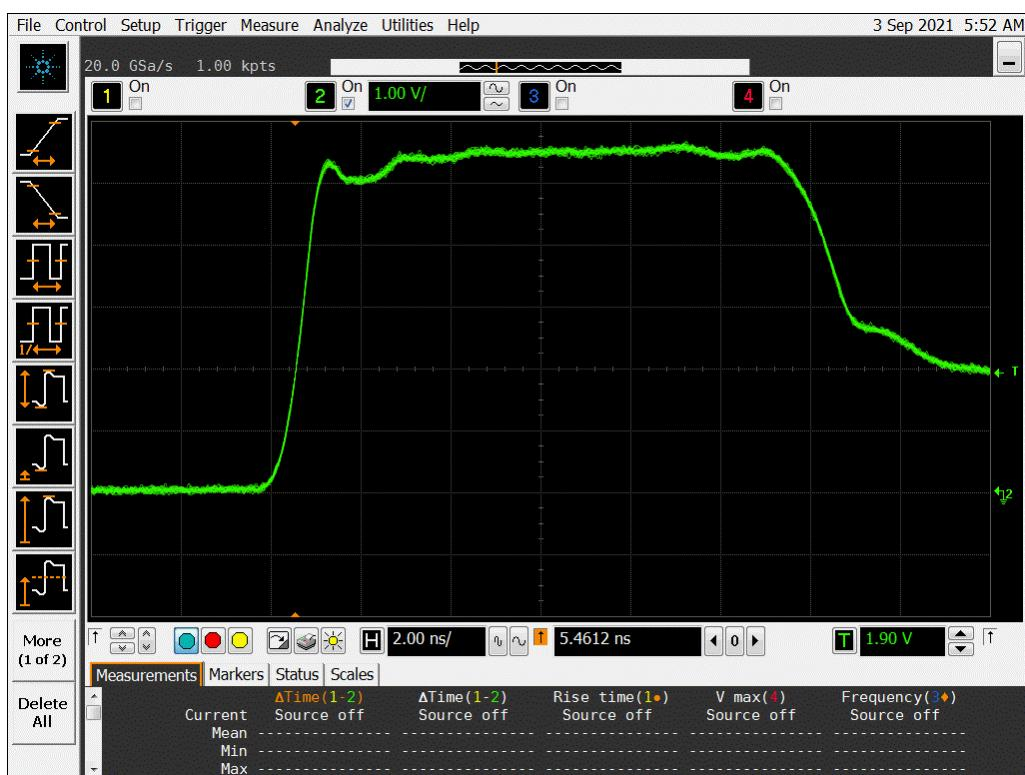
**Figure 10b DUT 2353 Post-Annealing Rising Edge**
