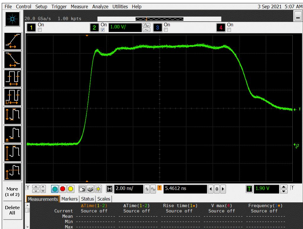
**Figure 14b DUT 2332 Post-Annealing Rising Edge**
