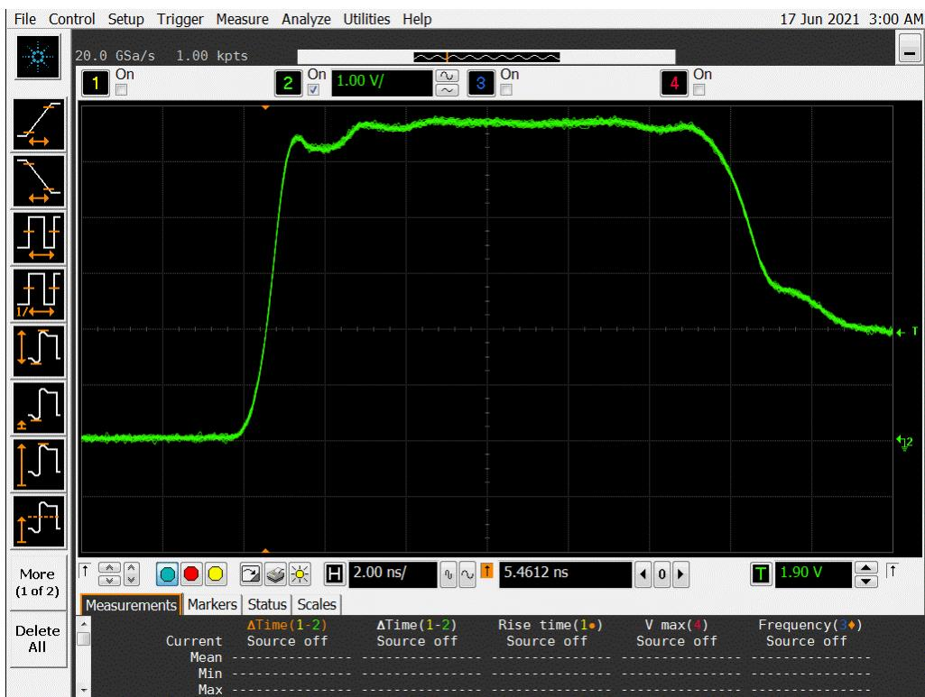
**Figure 14a DUT 2332 Pre-Irradiation Rising Edge**
