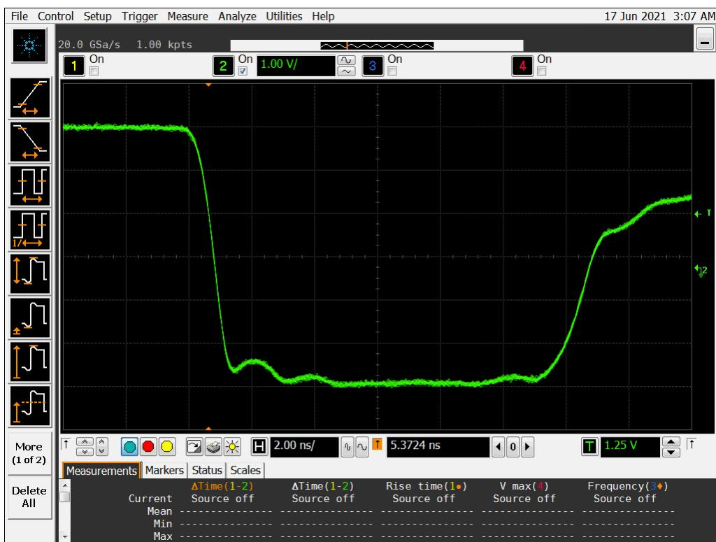
Figure 16a DUT 2353 Pre-Irradiation Falling Edge
