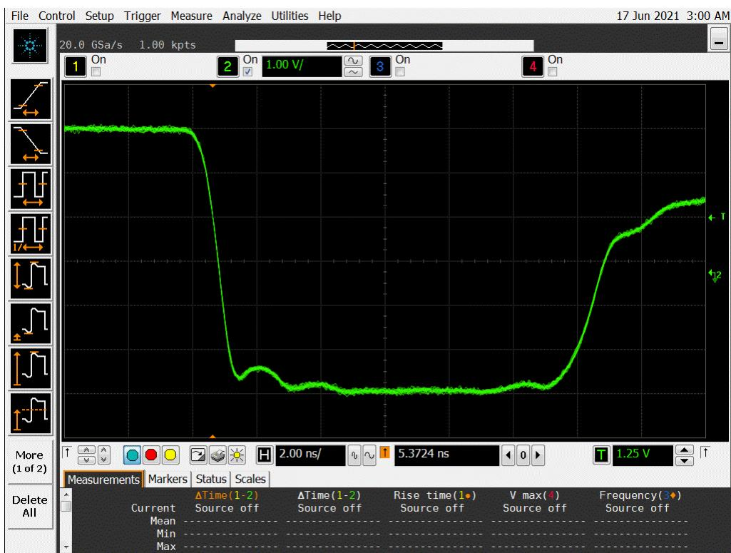
**Figure 20a DUT 2332 Pre-Irradiation Falling Edge**
