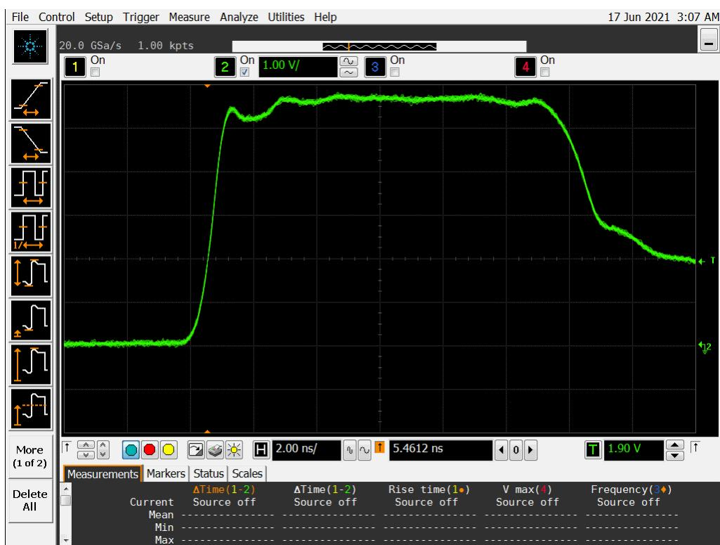
**Figure 10a DUT 2353 Pre-Irradiation Rising Edge**
