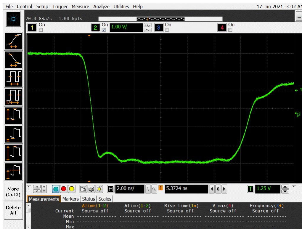
**Figure 17a DUT 2338 Pre-Irradiation Falling Edge**
