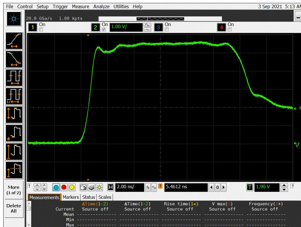
**Figure 11b DUT 2338 Post-Annealing Rising edge**
