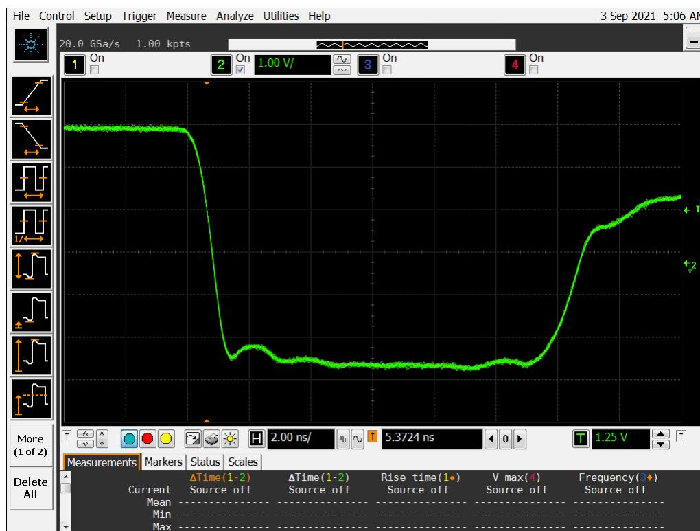
**Figure 19b DUT 2326 Post-Annealing Falling Edge**
