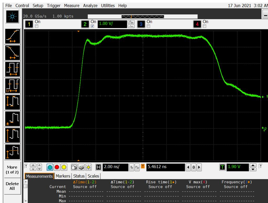
**Figure 11a DUT 2338 Pre-Radiation Rising Edge**
