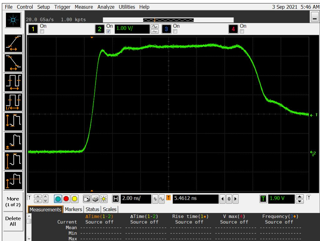
Figure 12b DUT 2342 Post-Annealing Rising Edge
