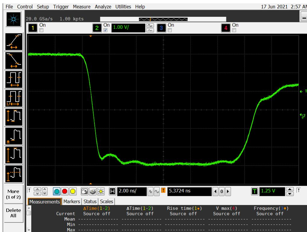
**Figure 19a DUT 2326 Pre-Irradiation Falling Edge**
