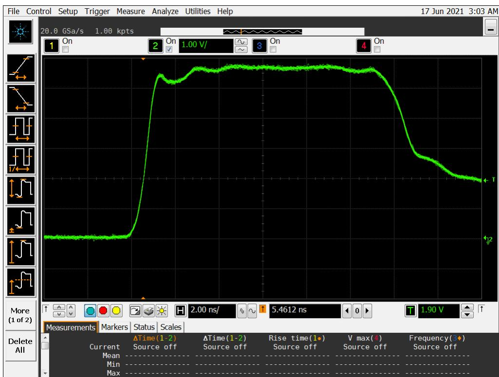
Figure 12a DUT 2342 Pre-Irradiation Rising Edge
