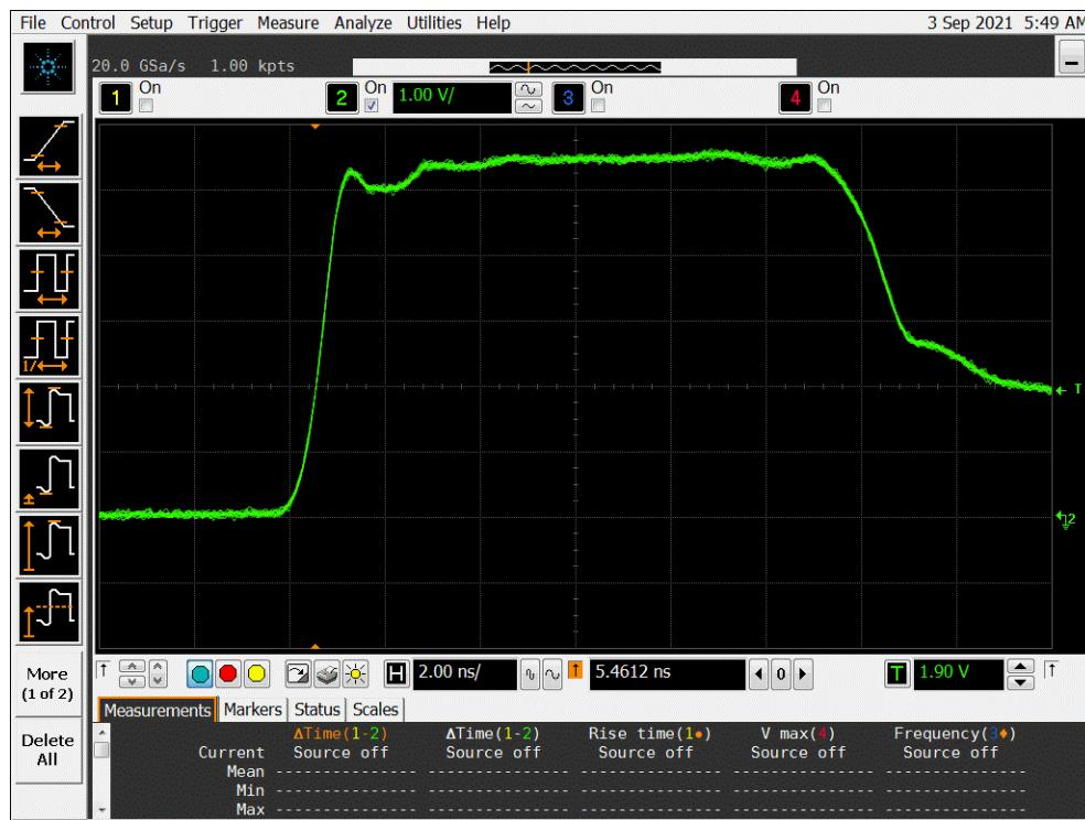
**Figure 9b DUT 2352 Post-Annealing Rising Edge**
