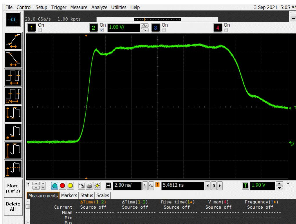
**Figure 13b DUT 2326 Post-Annealing Rising Edge**
