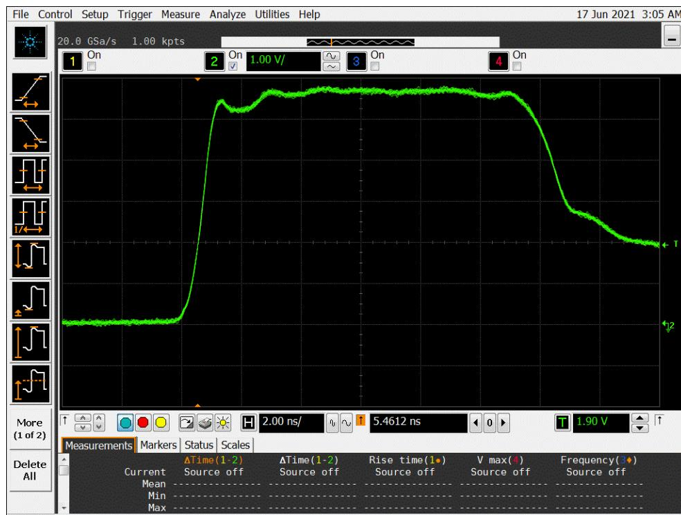
**Figure 9a DUT 2352 Pre-Irradiation Rising Edge**
