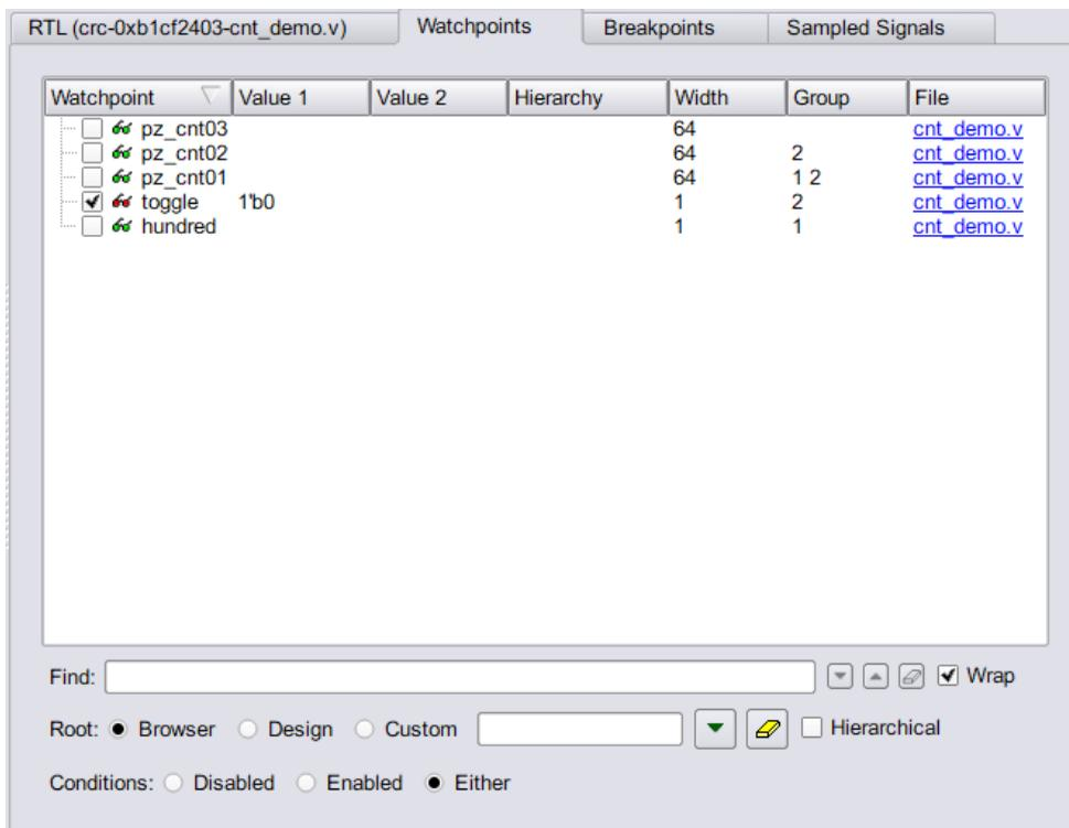
A watchpoint creates a trigger that is determined by the state of a signal in the design. The watchpoint can trigger either on the value of a signal or on a transition of a signal from one value to another.
