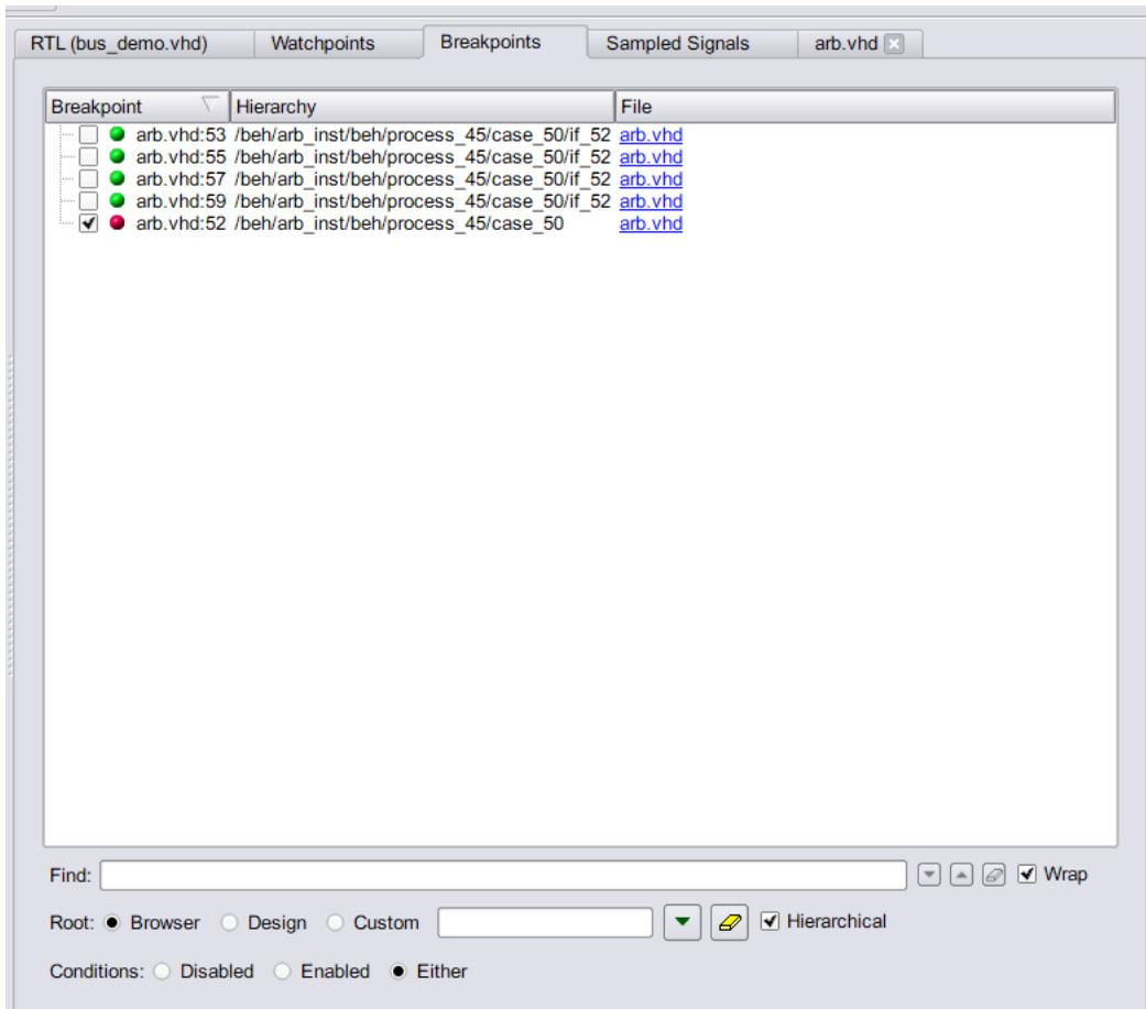
Breakpoints are a way to easily create a trigger that is determined by the flow of control in the design.
