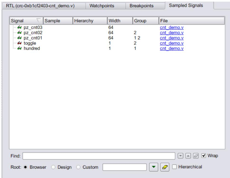
The sampling block is basically a large memory used to store all the sampled signals. During an active debugging session, the sampled signals are continually being stored in the sample block. When the sample block receives an event from the Master Trigger Signal event logic or the complex counter logic, the sampling block stops writing new data to the buffer and holds its contents. Eventually, the contents of the sample block are uploaded to the debugger for display and formatting.
