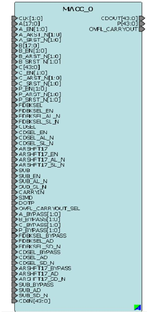
All signals of the SmartFusion2 MACC block, except CDIN and CDOUT, have optional registers. All registers must use the same clock. Each of the registers has enables and resets that can differ from each other. For a complete list of all the block options and their configurations, refer to the Microsemi documentation.
