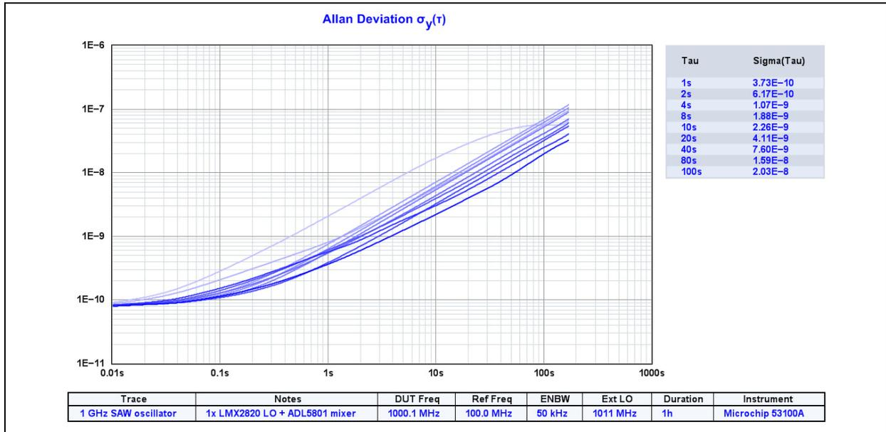
**FIGURE 14:** Dynamic Evolution of VCISO Frequency Stability During Warmup.
