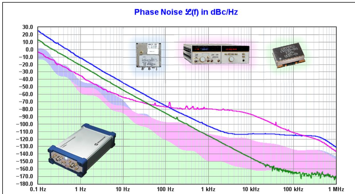
To measure signals at carrier frequencies beyond the 53100A's 200 MHz specification limit, it's necessary to transform UHF and microwave signals from the device under test (DUT) to a frequency within the 1 MHz to 200 MHz range. Two different strategies for accomplishing the necessary frequency transformation will be discussed in this application note: frequency division and heterodyne downconversion.
