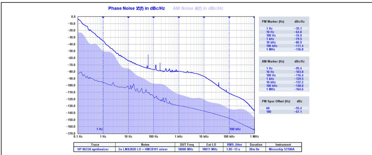
**FIGURE 21:** Phase Noise, AM Noise, and Jitter of Commercial Microwave Synthesizer, Measured with Dual-Channel Downconverter.
