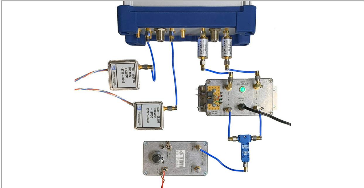
**FIGURE 5:** (Counterclockwise from Top) Microchip 53100A, Dual 100 MHz Reference Oscillators, 1000 MHz SAW Oscillator Module (DUT), Microwave Power Splitter, Dual HMC983 Divider Module, 21.4 MHz Lowpass Filters (Mini-Circuits SLP-21.4).
