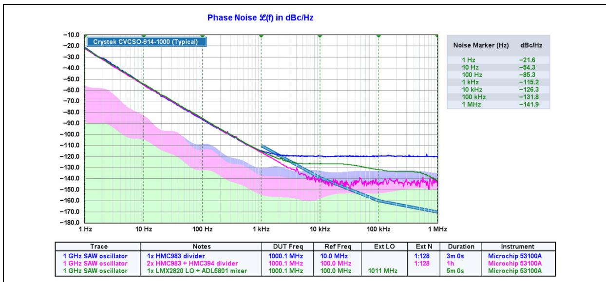
**FIGURE 15:** VCSO Phase Noise Measurement with Single-Channel Downconverter (Green Trace).
