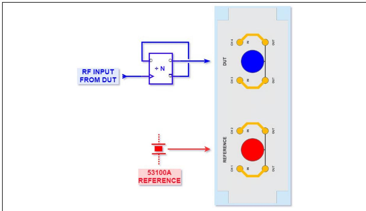
**FIGURE 1:** Basic Measurement Setup for Frequency Division. The D Flip-Flop Represents an Arbitrary Division of the DUT Frequency by N.
