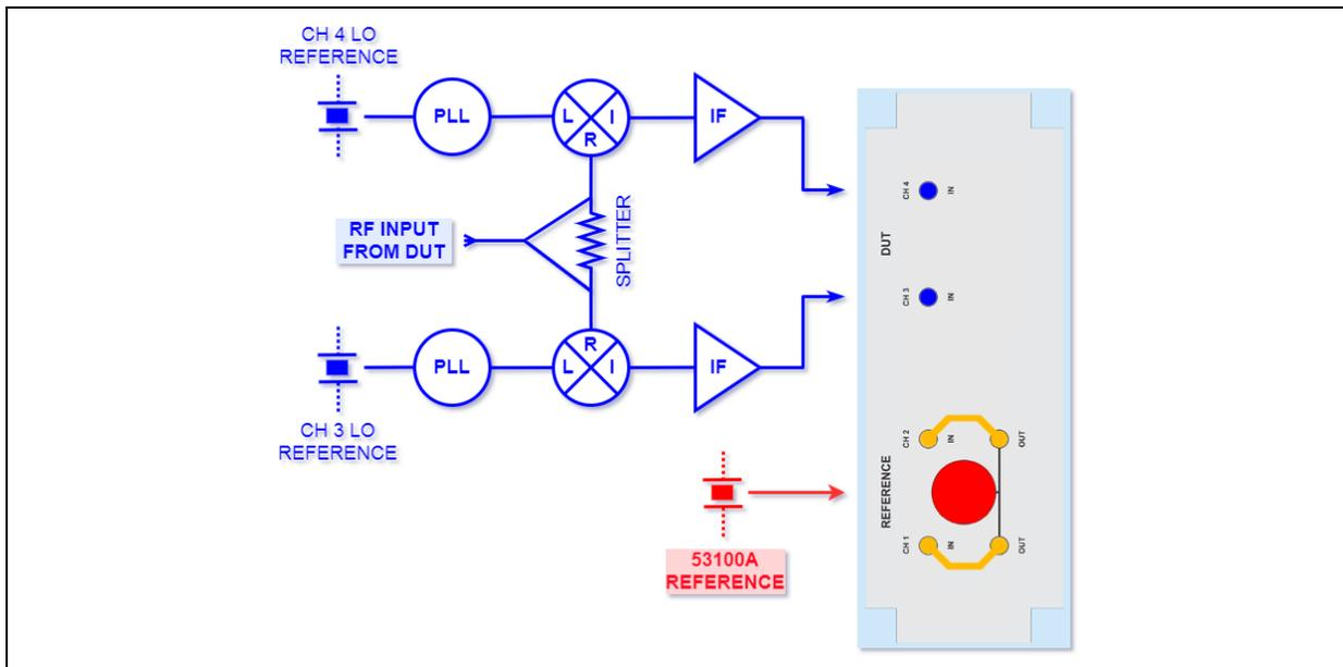
**FIGURE 16:** Dual-Channel Downconverter Block Diagram.
