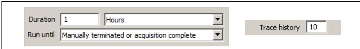
**FIGURE 11:** Setting the Measurement Duration and Allan Deviation Trace History Count.
