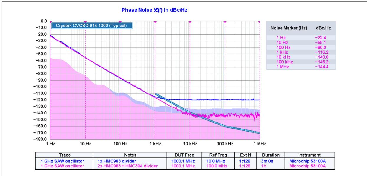
**FIGURE 6:** Result of Cross-Correlated Measurement with Two Frequency Dividers.
