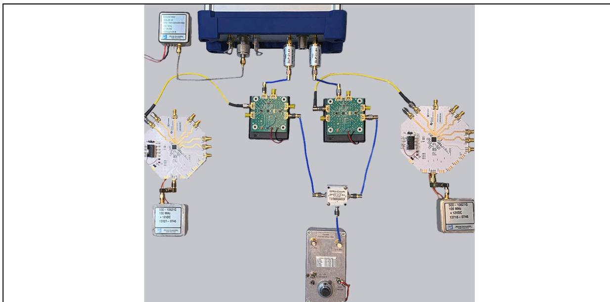
**FIGURE 17:** Dual-Channel Downconverter Test Hardware.
