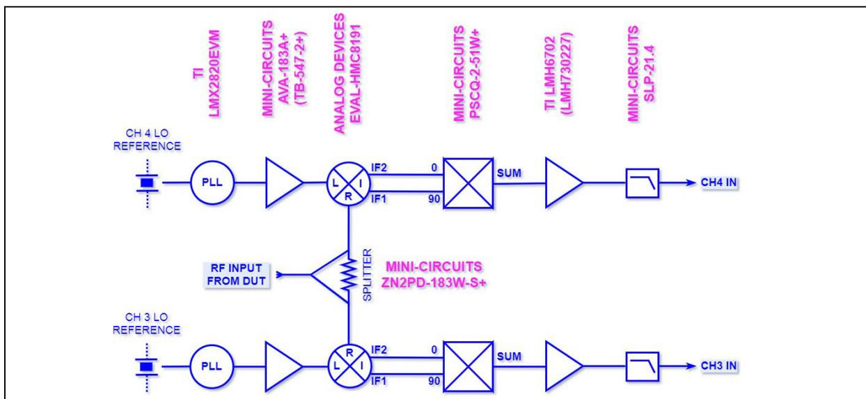
**FIGURE 19:** Example Block Diagram for 6 GHz to 18 GHz Dual-Channel Downconverter.
