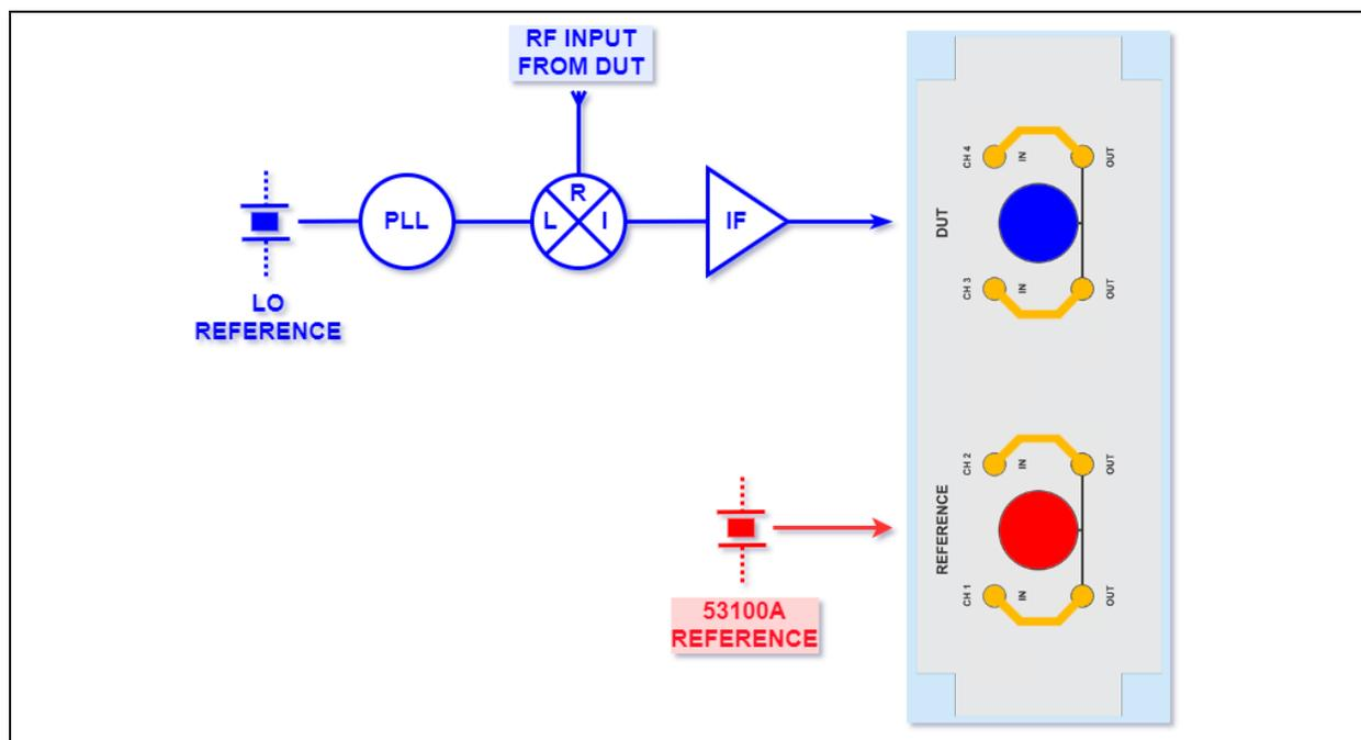
**FIGURE 7:** Downconverter Block Diagram Showing Connections to Microchip 53100A Front Panel.
