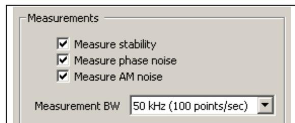
**FIGURE 10:** Increasing the Stability Measurement Bandwidth.
