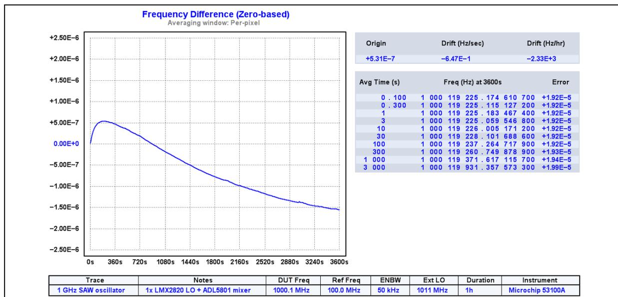
**FIGURE 13:** 1000 MHz VCISO Frequency Drift Shortly after Power-On.
