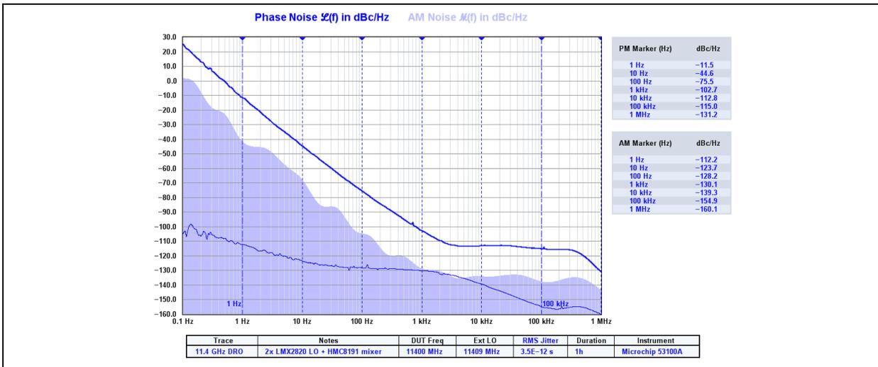
**FIGURE 20:** Phase Noise, AM Noise, and Jitter of 11.4 GHz Dielectric Resonant Oscillator (DRO), Measured with Dual-Channel Microwave Downconverter.
