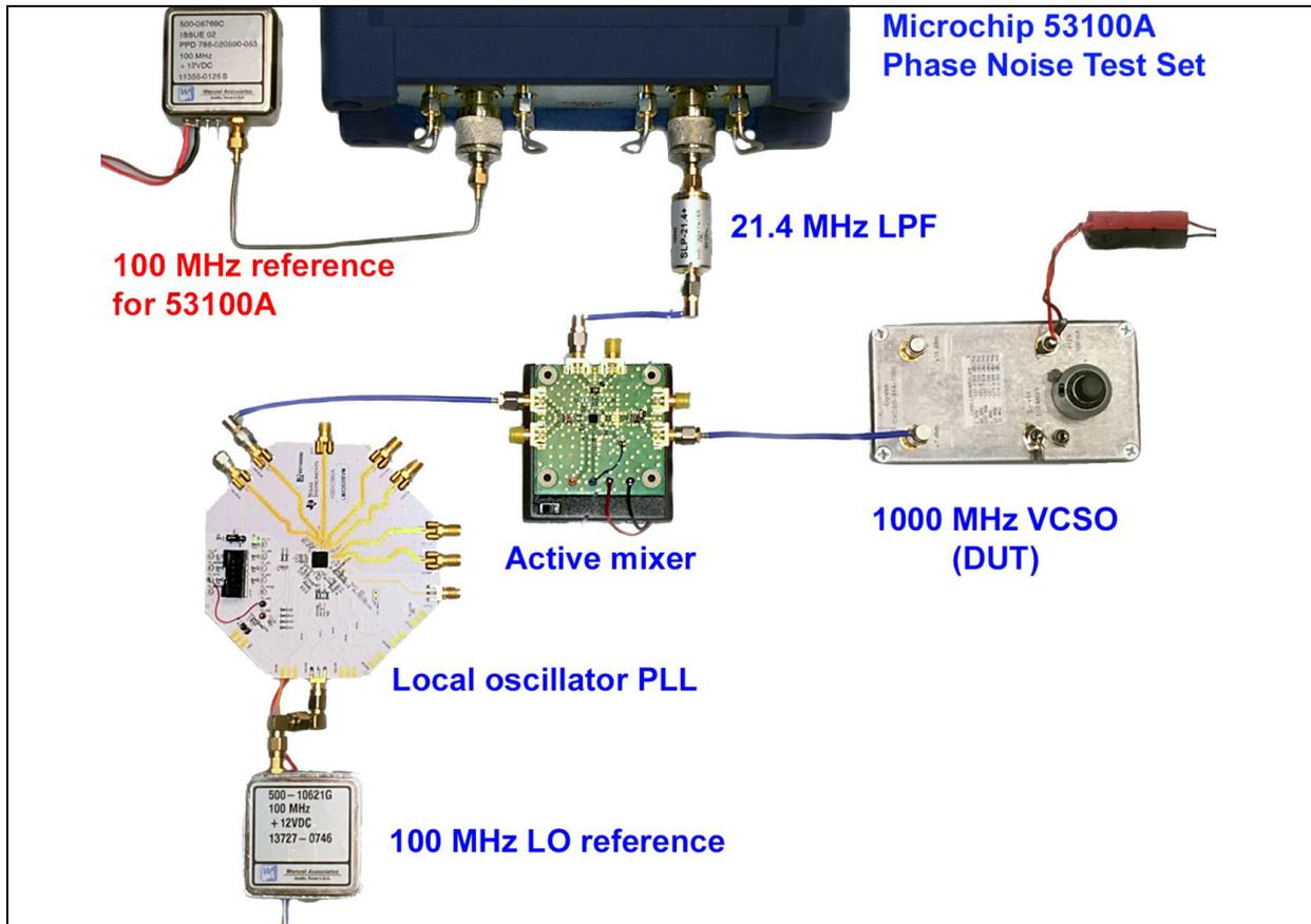
**FIGURE 8:** Single-Channel Heterodyne Downconversion with LO and Mixer Capable of 6000 MHz Operation.
