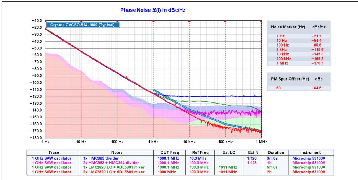
**FIGURE 18:** VCSO Measurement with Dual-Channel Downconversion (Red Trace) Compared to Previous Results.
