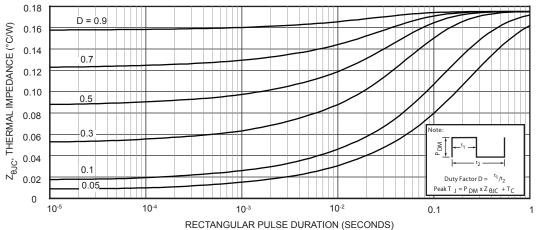
RECTANGULAR PULSE DURATION (SECONDS) Figure 3b, Maximum Effective Transient Thermal Impedance, Junction-To-Case vs Pulse Duration
