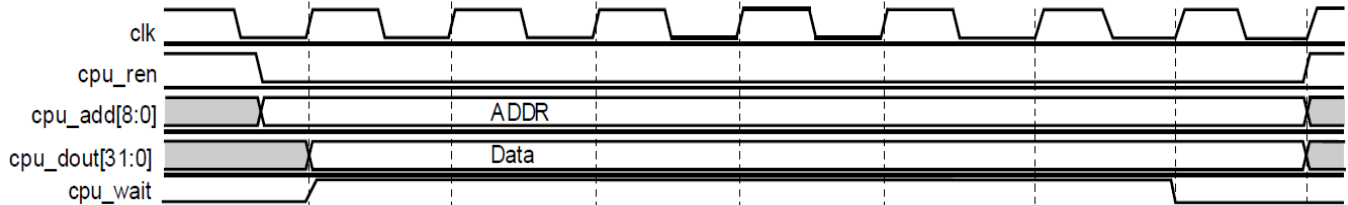
Figure 9 CPU Interface Control/Status Register Read Cycle
