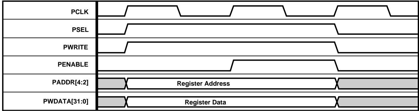
Figure 3 Data Write Cycle
