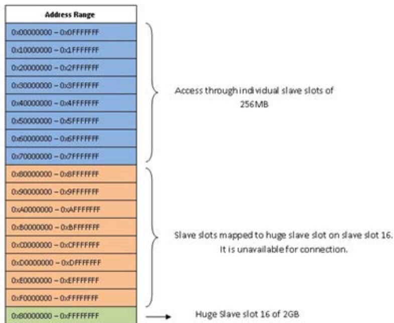
Figure 15 . Memory Map when Memory space is Set to 8 Slots of 256 MB and 1 Huge Slot of 2 GB Beginning at Address 0x80000000
