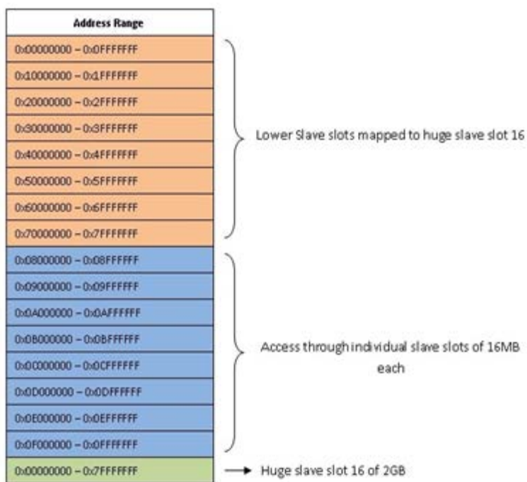
Figure 16 . Memory Map when Memory Space is Set to 8 Slots of 16 MB and 1 Huge Slot of 2 GB, Beginning at Address 0x00000000 to 0x7FFFFFFF
