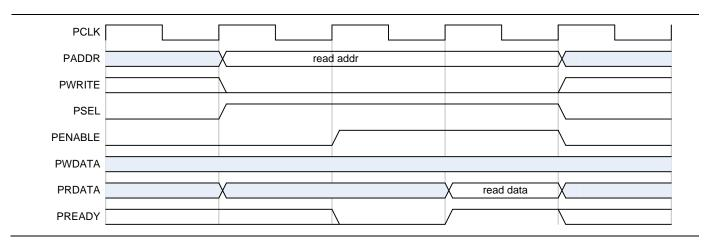
Figure 7 APB Read Transfer with One State
