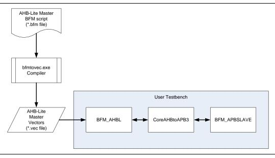
Figure 10 CoreAHBtoAPB3 User Testbench
