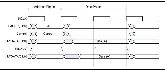
Figure 3 AHB Transfer with One Wait State
