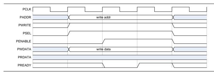
Figure 6 APB Write Transfer with One State
