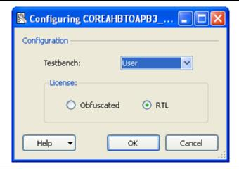
Figure 8 CoreAHBtoAPB3 Configuration GUI
