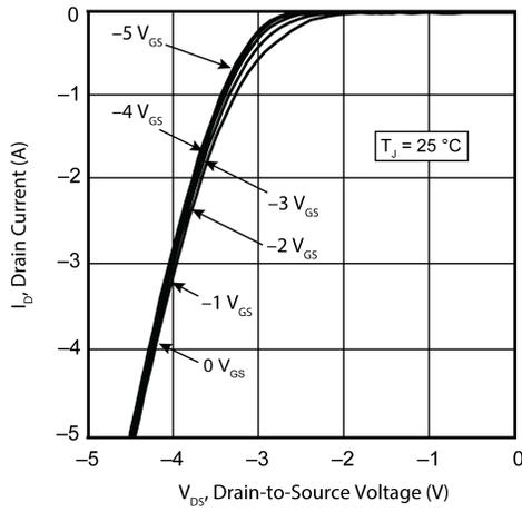
Figure 9 •  $I_D$  vs.  $V_{DS}$  3<sup>rd</sup> Quadrant Conduction
