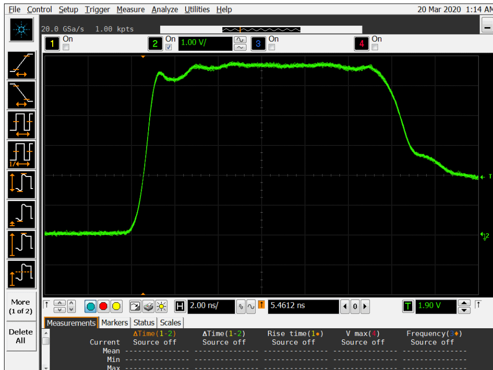
Figure 9b DUT 14063 Post-Annealing Rising Edge
