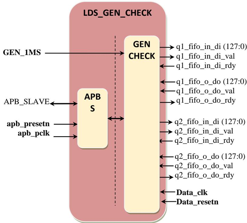
The goal of this module is to generate a counter when writing to the disk and checking the value received when reading the disk.
