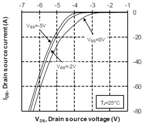
**Figure 13 • 3<sup>rd</sup> Quadrant Characteristics, TJ = 25 °C**
