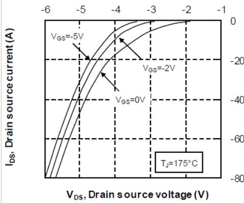
Figure 15 • 3<sup>rd</sup> Quadrant Characteristics,  $T_J = 175^\circ\text{C}$
